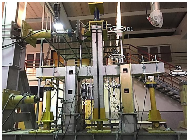
Figure 10. Testing set up, loading system and location of potentiometers (D's are potentiometers)
