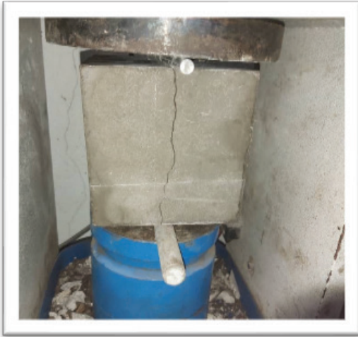
Figure 3. Brazilian tensile strength test on C350F and C350.
