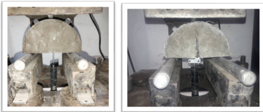
Figure 5. Failure of fiber-reinforced specimen in SCB test.
