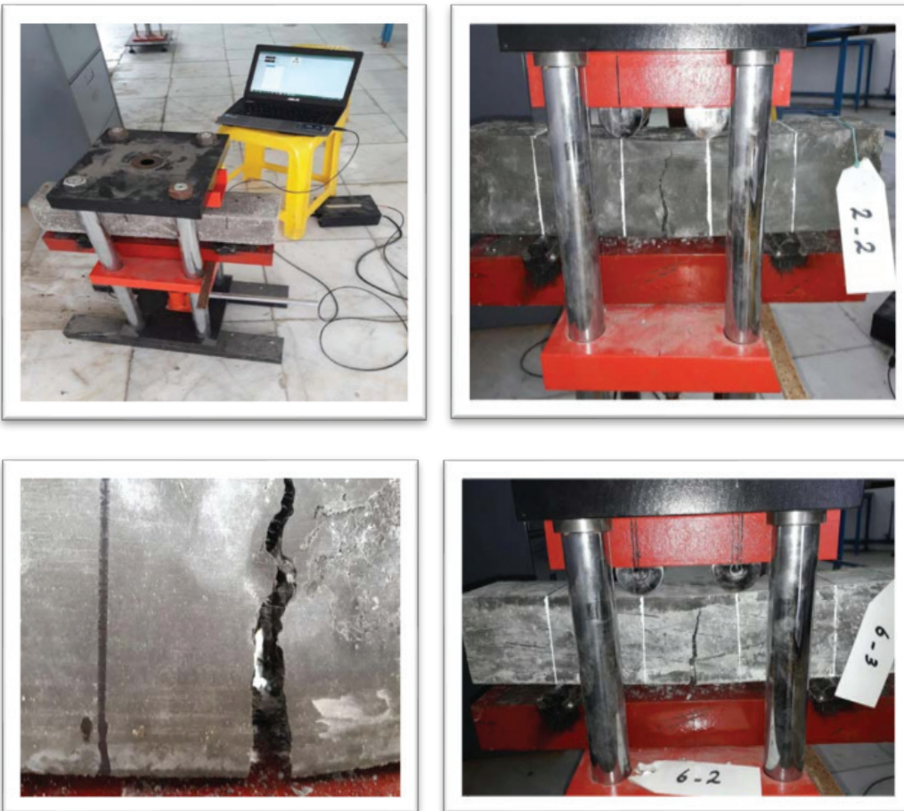
Figure 4. Specimen failure mode in the flexural strength test.
