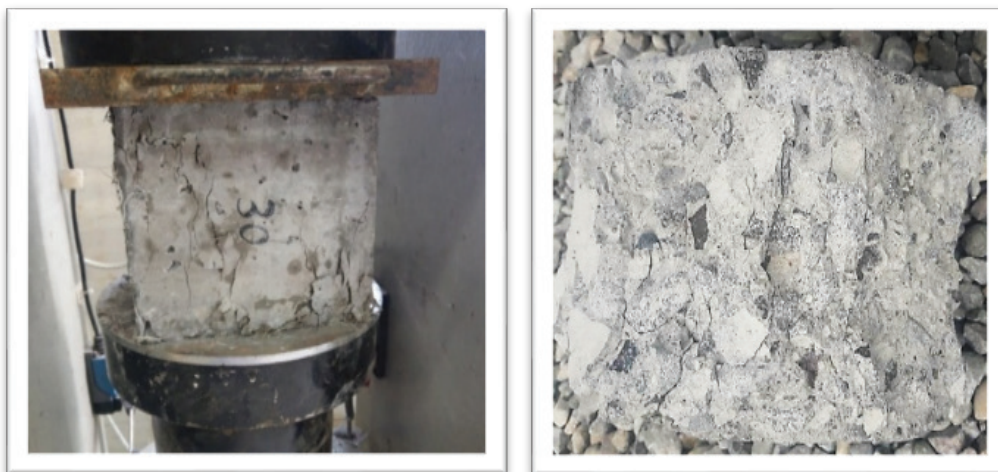
Figure 2. Specimens C350 and C350F after the compressive strength test.
