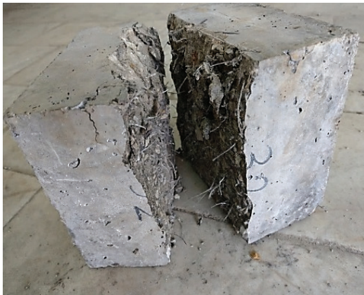
Figure 7. Fractured specimen after SCB test, showing fiber bridging and crack resistance due to Forta-Ferro fibers.
