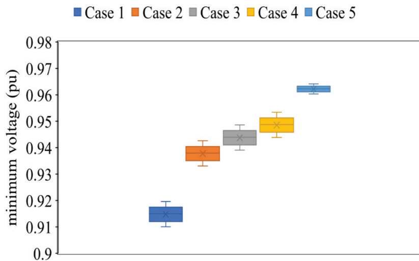
Figure 13. Sensitivity analysis of minimum voltage of the system under cases for 33 bus system.
