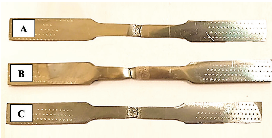
Figure 8. Tensile test samples fracture location (A) 100 A, (B) 150 A, and (C) 190 A.
