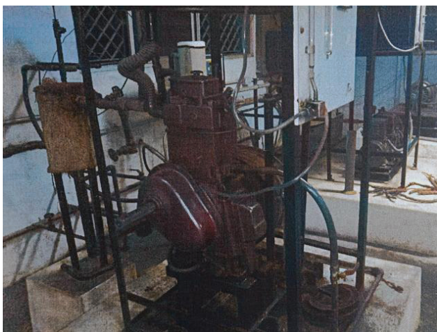
Figure 2(a). Experimental setup: four stroke, 5 H.P single cylinder diesel engine. (It was drawn by the author).
