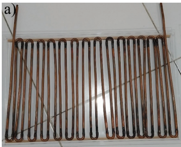
Figure 1. a) Photograph of serpentine tube and b) Dimension of the PVTC unit.
