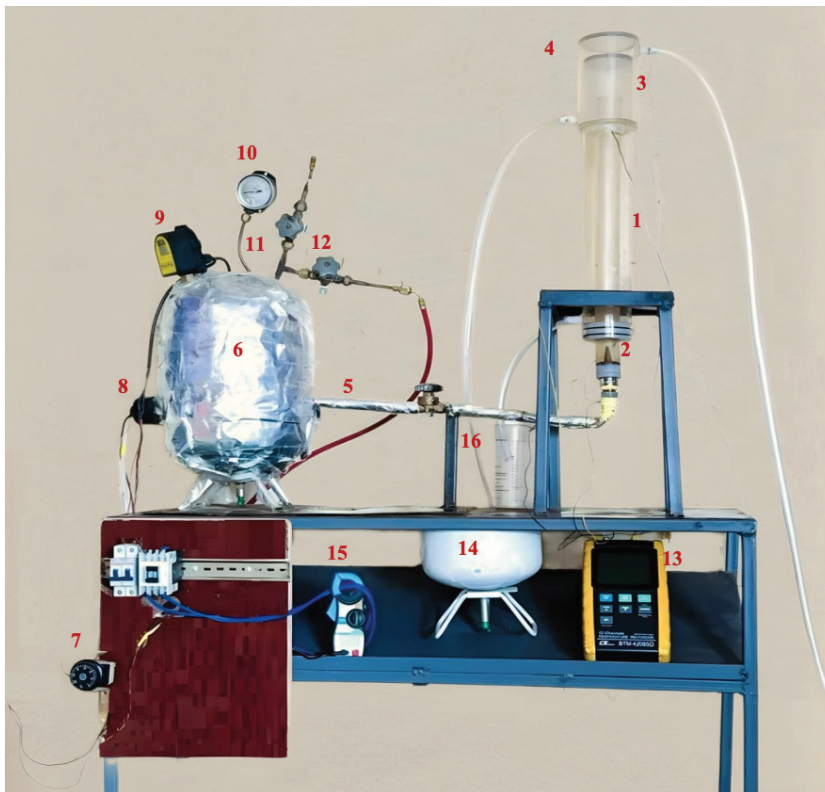
Figure 4. Complete experimental testing device: (1) Heat pipe (2) Nozzle (3) Condenser (4) Water jacket (5) Connecting pipe (6) Water tank (7) Control panel (8) Electrical heater (9) Digital pressure valve (10) Pressure valve (11) Pressure safety valve (12) Control valve (13) Data logger (14) Charging storage (15) Clamp meter (16) Condensate storage.
