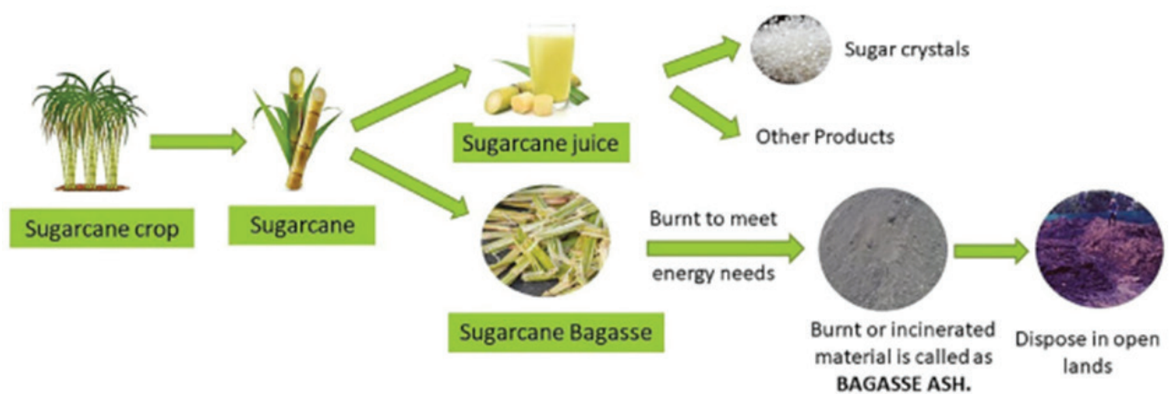
Figure 2. The processing of sugarcane bagasse ash [From Khandelwal [15], retrieved from Elsevier. Open access and property citation has been done..
