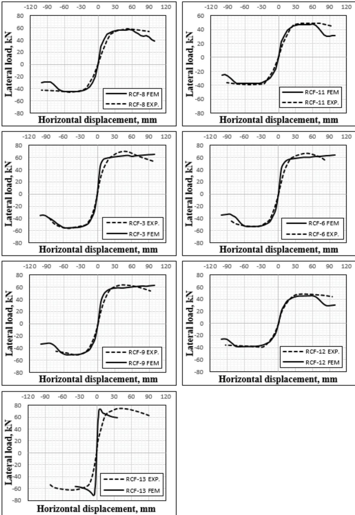
Figure 22. Comparison of strength envelope curves of reinforced concrete frame elements .
