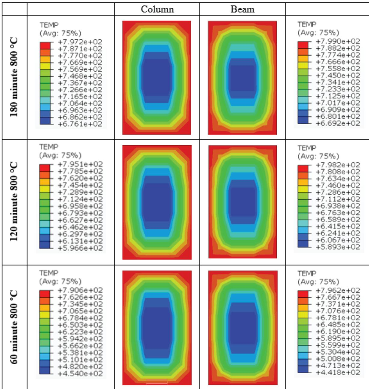
Figure 16. Heat transfer study for a reinforced concrete frame sample where 800°C temperature is applied for 60, 120 and 180 minutes.
