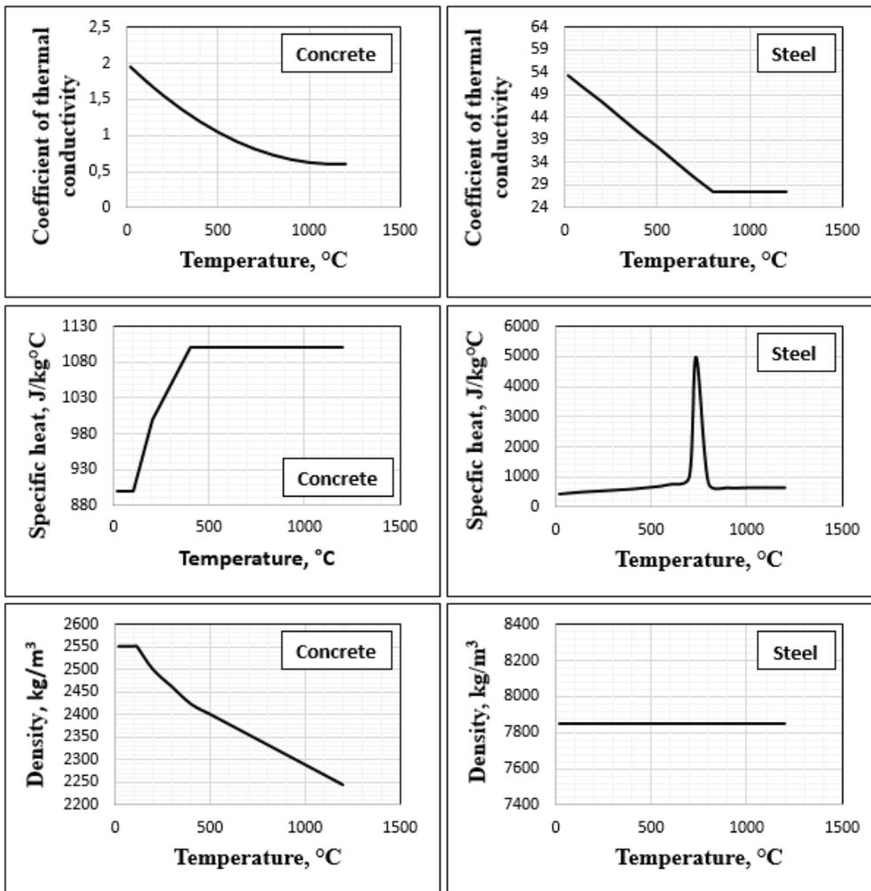
Figure 6. Basic thermal properties for concrete and steel.
