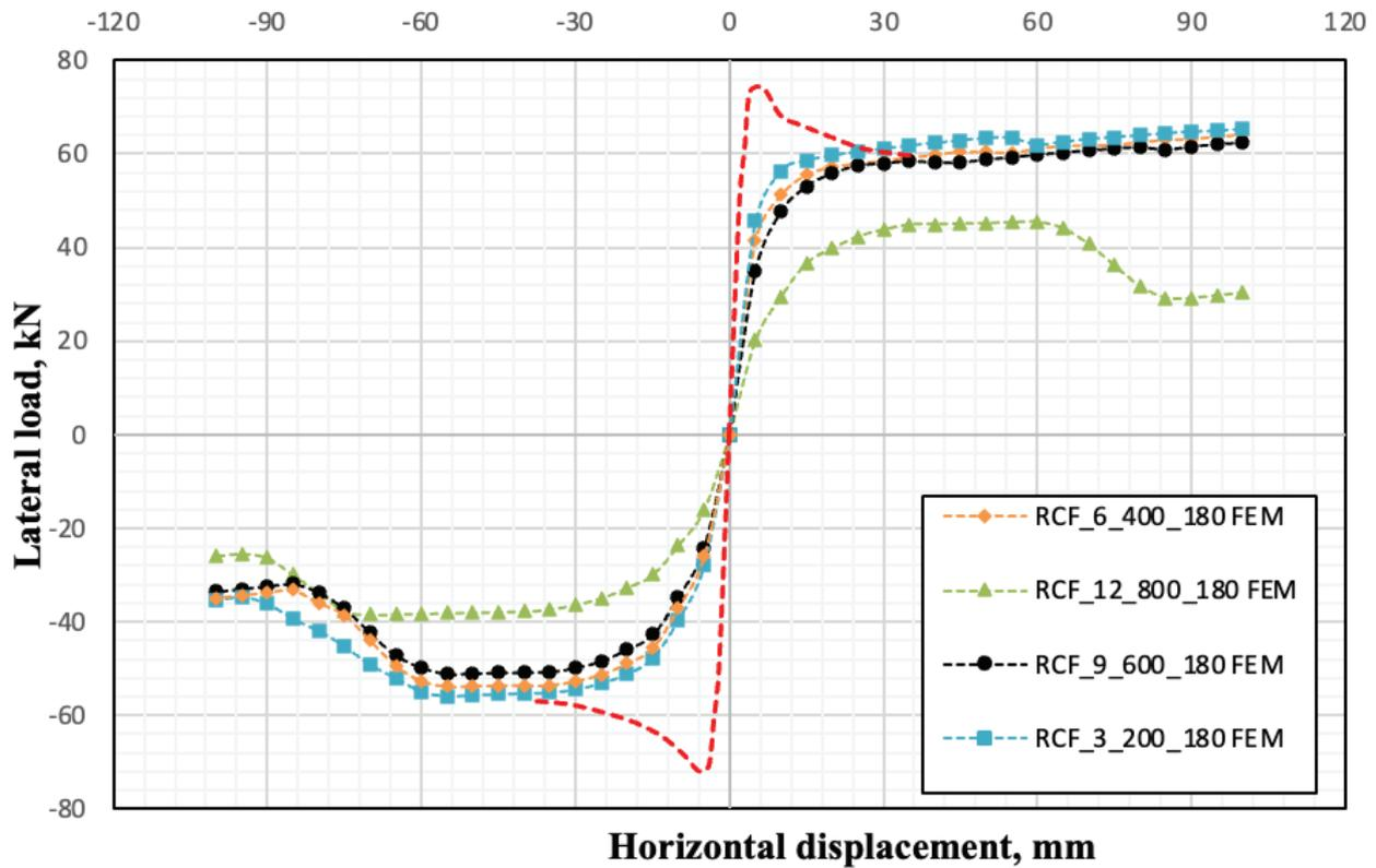
Figure 19. Strength envelope curves (180 minute).
