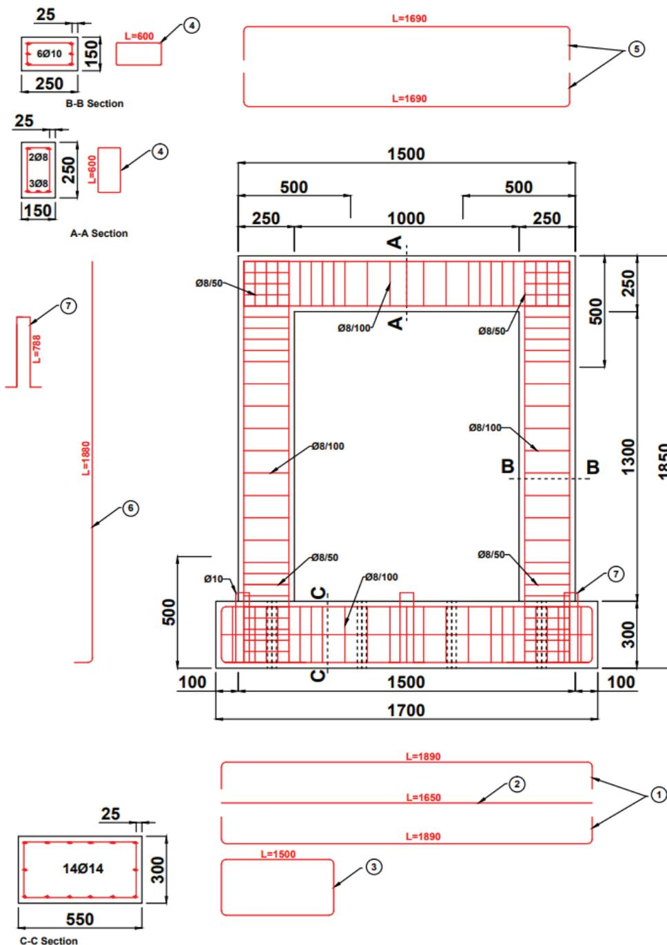
**Figure 2.** Reinforcement properties of reinforced concrete frame elements.
