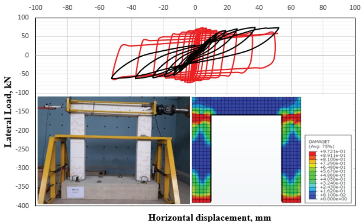
Figure 3. Determining the reliability of the finite element modelling method.
