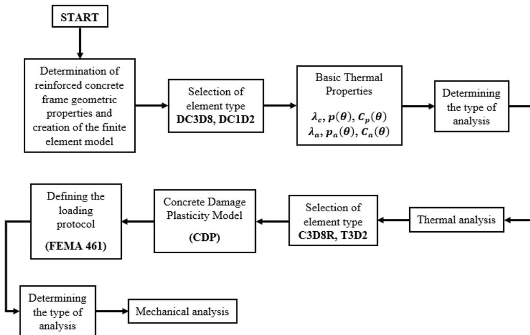
**Figure 4.** The process of evaluating the cyclic lateral load performance of reinforced concrete frames after high temperature.
