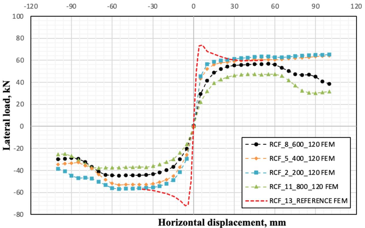
Figure 18. Strength envelope curves (120 minute).
