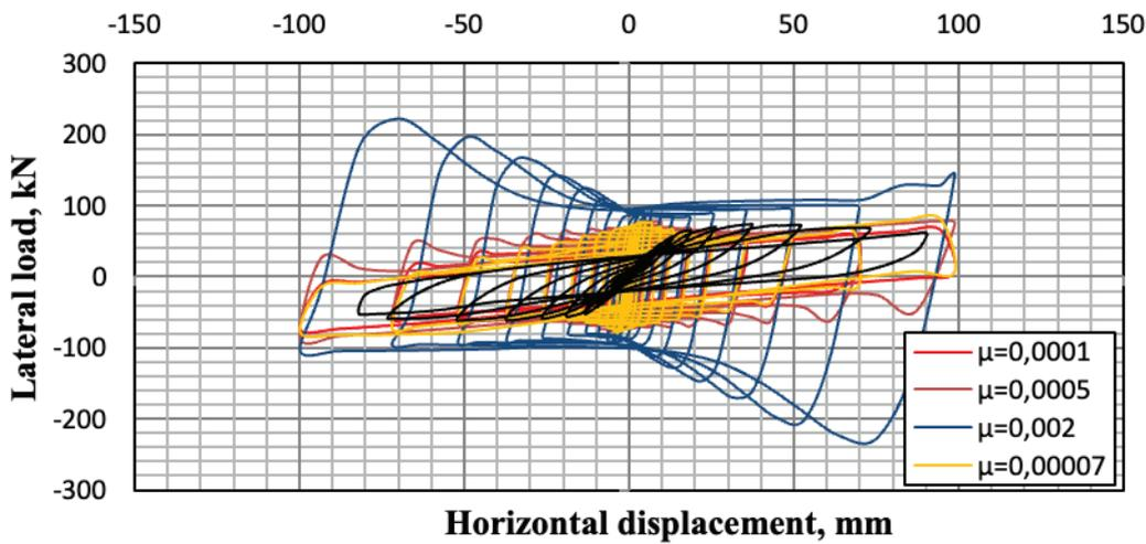
Figure 12. Effect of viscosity change on lateral load - horizontal displacement relationship.
