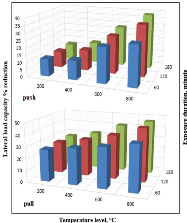
Figure 20. Lateral load carrying capacity - temperature relationship.
