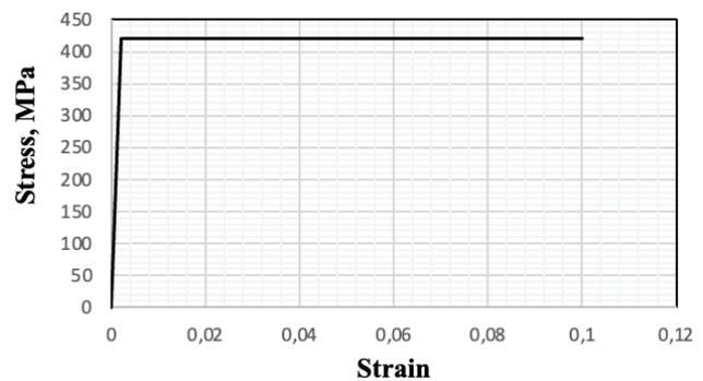
Figure 13. Stress – strain relationship of steel reinforcement.
