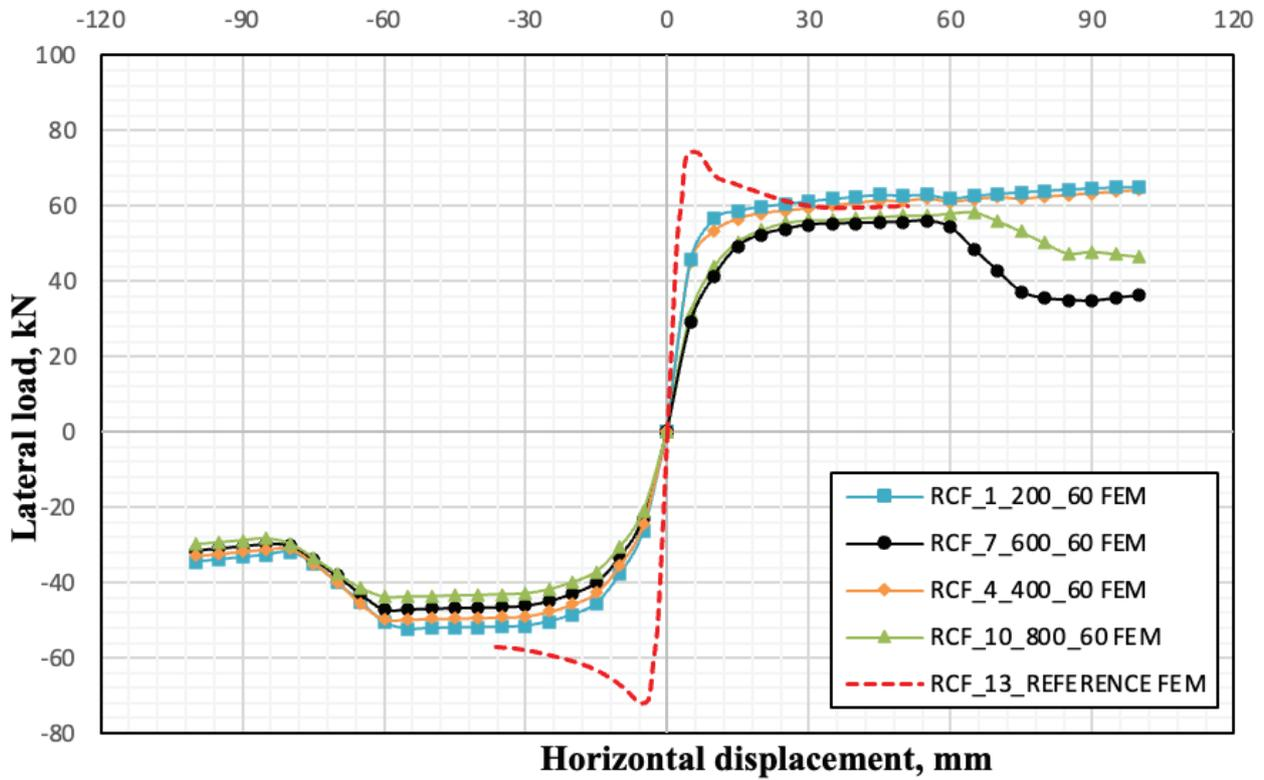
Figure 17. Strength envelope curves (60 minute).
