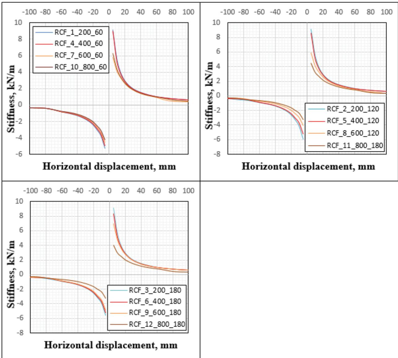
Figure 21. Change of stiffness – lateral displacement relationship with temperature.
