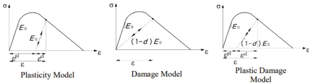
Figure 8. Relationship between damage and plasticity.
