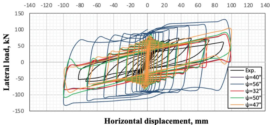
Figure 11. Effect of change of dilation angle on lateral load - horizontal displacement relationship.
