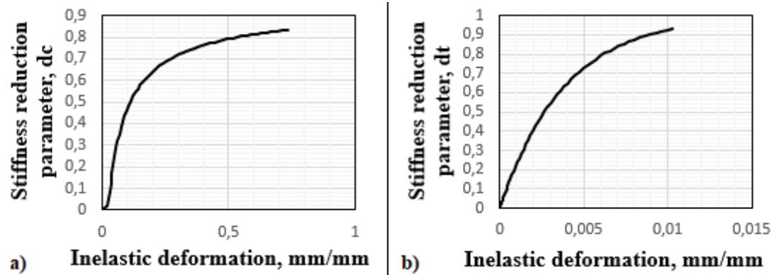
Figure 10. Change of stiffness reduction parameter due to inelastic deformation a) for compression b) for tension.
