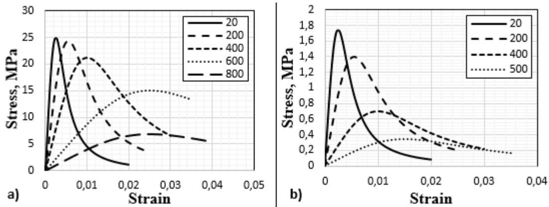
Figure 9. Idealized stress – strain curves of concrete a) For axial compression b) For axial tension.
