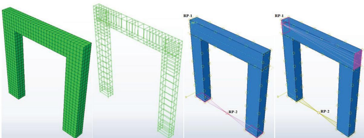
**Figure 5.** Finite element model of reinforced concrete frame test elements.
