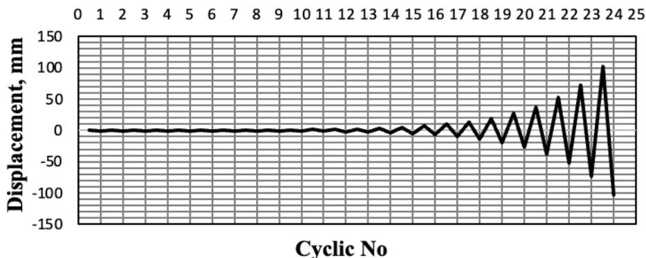
Figure 15. Cyclic lateral loading protocol.
