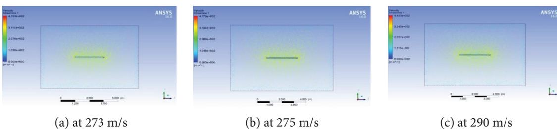
**Figure 17.** Wing without winglets under unsteady transonic flow.
