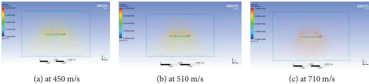
Figure 21. Wing with sharp-edge multi-winglets under unsteady supersonic flow.
