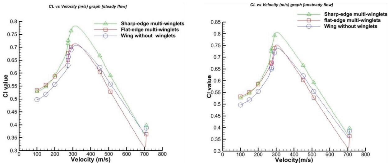
**Figure 3.** (a) Cl vs velocity variation under steady flow
