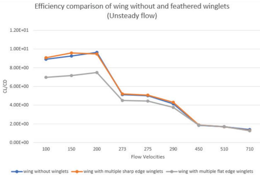
Figure 24. Comparison of wing with Feathered winglets and wing without winglets in unsteady flow.
