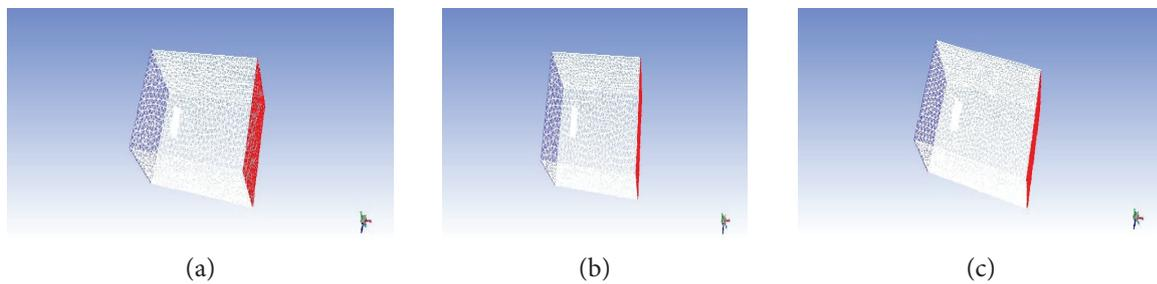
**Figure 2.** (a) Meshing of wing without winglets (b) Meshing of wing with sharp-edge winglets (c) Meshing of wing with sharp-edge winglets.
