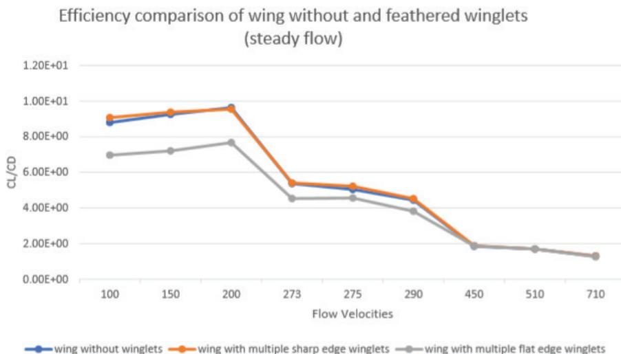
Figure 23. Comparison of wing with Feathered winglets and wing without winglets in steady flow.
