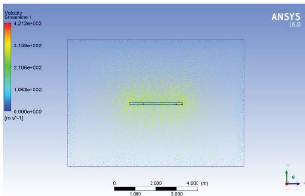
Figure 9. Wing without winglets under transonic flow at 273 m/s
