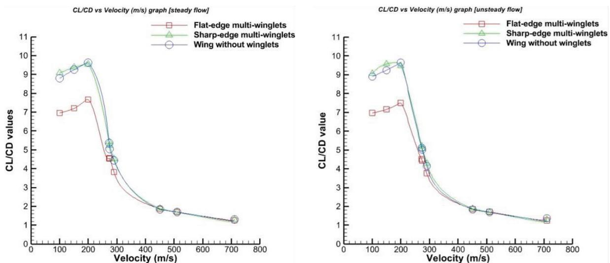
Figure 5. (a) CL/CD vs velocity max graph (steady flow) b) CL/CD vs velocity max graph (unsteady flow)
