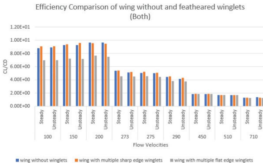
**Figure 25.** Efficiency comparison of steady and unsteady flow of wing without and wing with feathered winglets.
