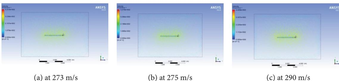
**Figure 18.** Wing with sharp-edge multi-winglets under unsteady transonic flow.
