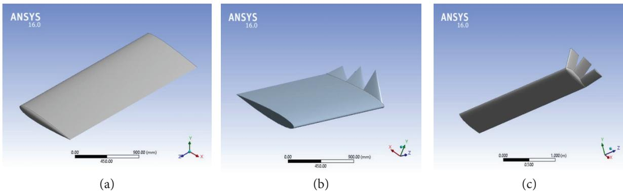
**Figure 1.** (a) Wing without winglets (b) Wing with sharp-edge multi-winglets (c) Wing with flat-edge multi-winglets.
