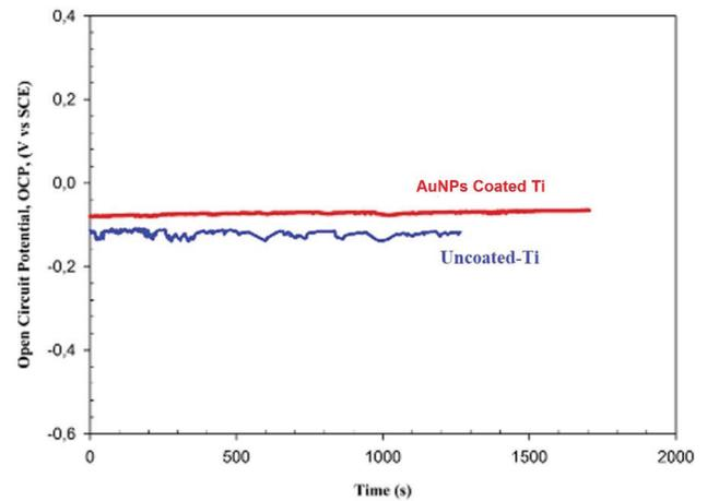
**Figure 5.** Open-circuit corrosion potential versus time of immersion in artificial saliva of the a) uncoated Ti, b) AuNPs-Coated Ti discs.
