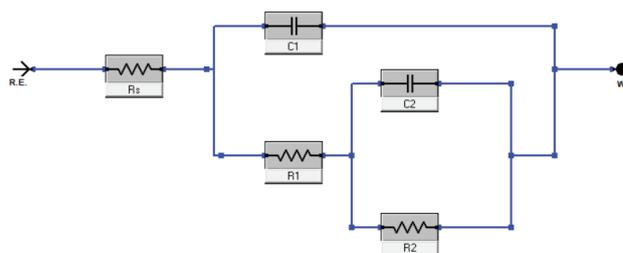
**Figure 9.** Equivalent electrical circuit for EIS data.
