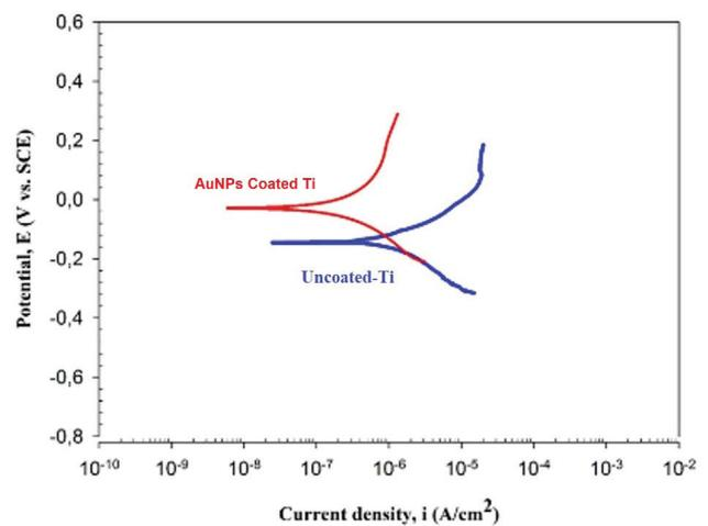
**Figure 6.** Tafel curves of the uncoated Ti and AuNPs-Coated Ti discs.
