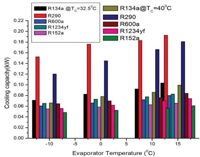
Figure 4. Cooling capacity vs. Evaporator temperature without LSHX.
