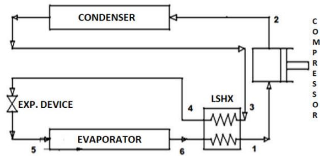
Figure 1. a) Refrigerator Test Rig, b) Schematic diagram.
