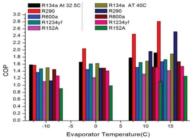
Figure 7. COP vs. Evaporator temperature with LSHX.
