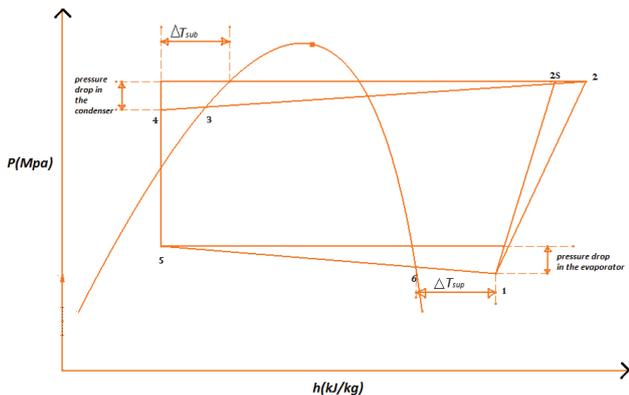
Figure 2. Pressure-enthalpy diagram.
