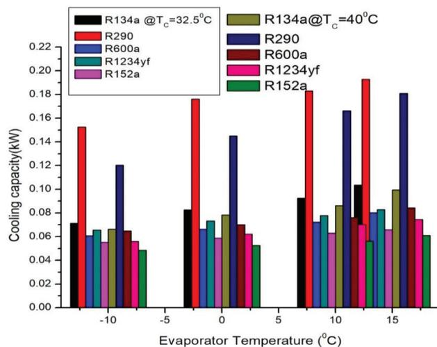
Figure 3. Cooling capacity vs. Evaporator temperature with LSHX.
