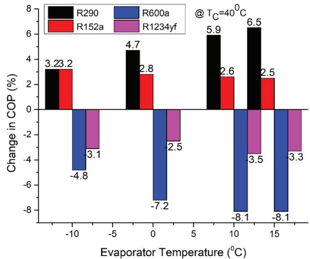
Figure 10. Change in COP (%) vs. Evaporator Temperature (Tc= 40°C).
