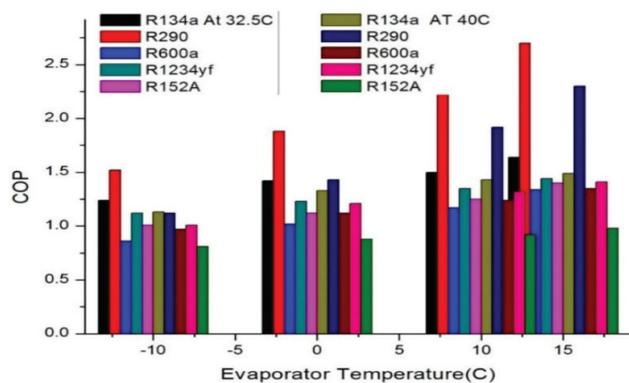
Figure 8. COP vs. Evaporator temperature without LSHX.
