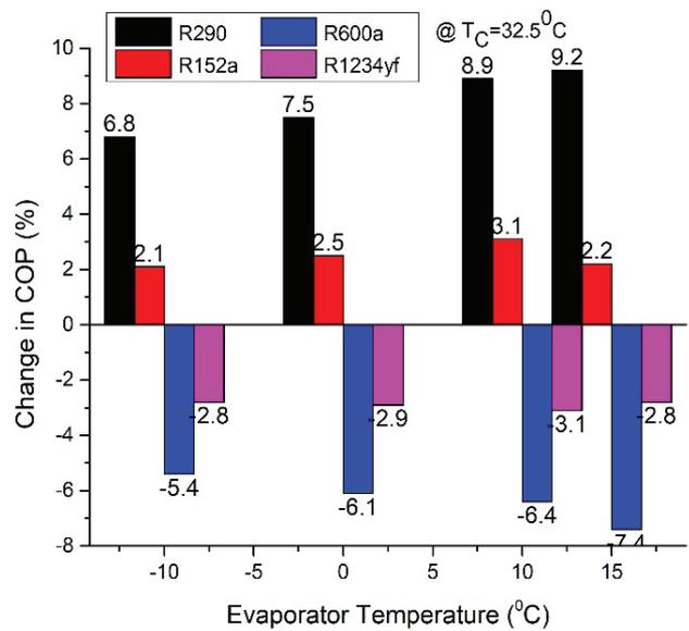
Figure 9. Change in COP (%) vs. Evaporator temperature (Tc= 32.5°C).
