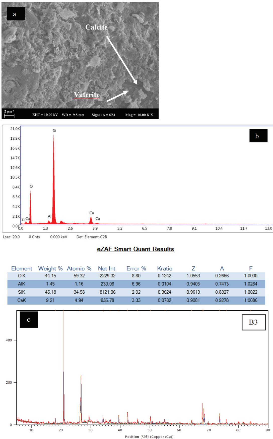
Figure 9. SEM micrograph of the B3 specimen a) 10,000 X SEM b) EDS c) XRD Analysis.
