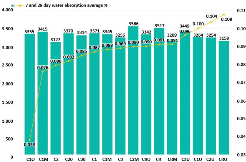
Figure 4. Water absorption -UPV test results of 0.6 w/c.
