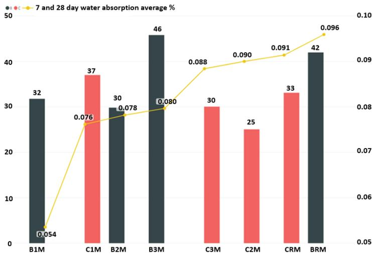
Figure 6. Water absorption-Compressive strength test results of the 0.5-w/c specimens containing metakaolin.
