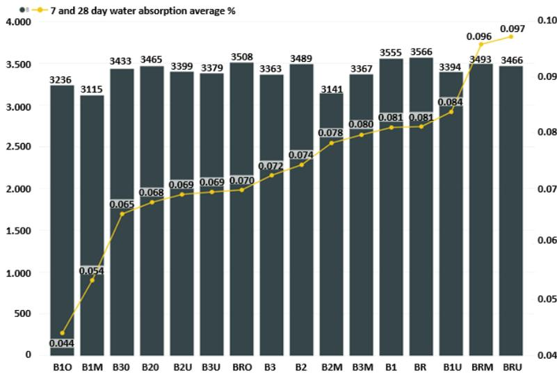
Figure 3. Water absorption and UPV test results of 0.5 w/c.
