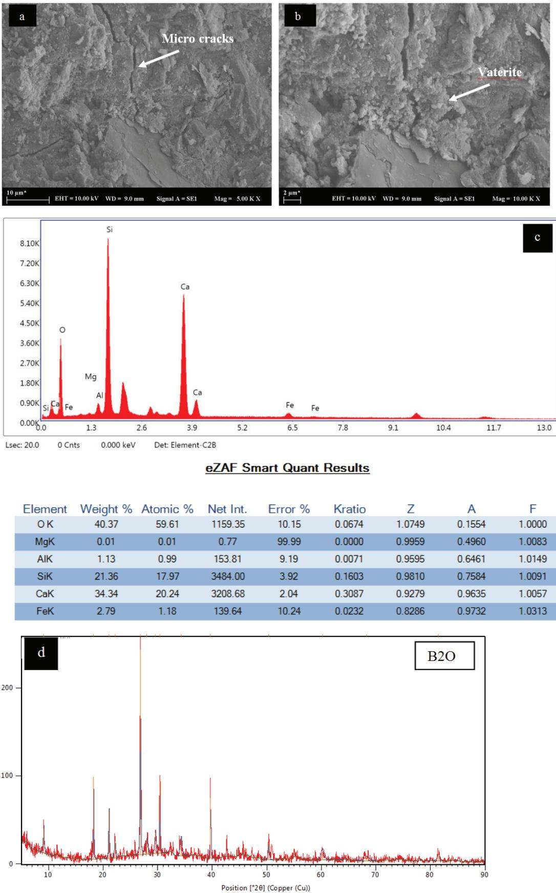
Figure 10. SEM micrographs of the B2O specimen a) 5000 X SEM b) 10,000 X SEM c) EDS d) XRD Analysis.
