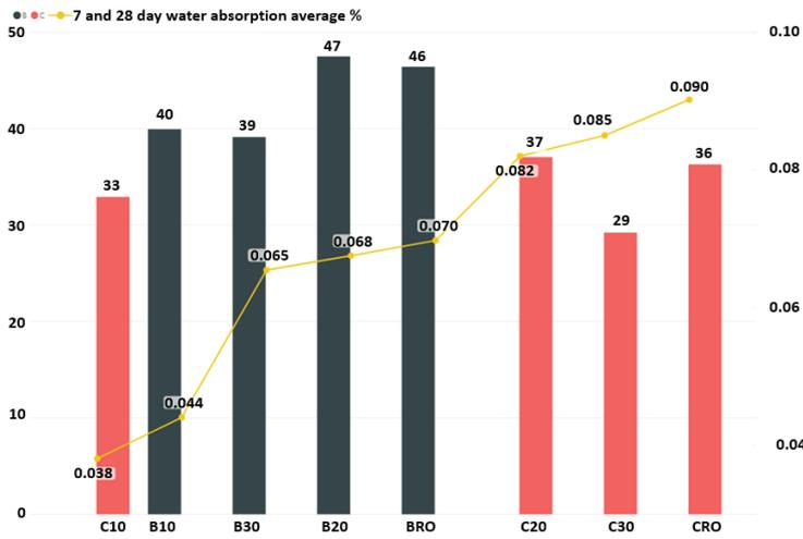
Figure 5. Water absorption-Compressive strength test results of the specimens containing GBFS.
