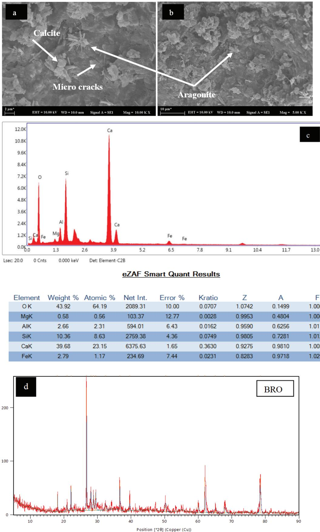
Figure 8. a) 5,000 X SEM b) 10,000 X SEM c) EDS d) XRD Analyses Results in the control specimen (BRO) SEM micrographs.
