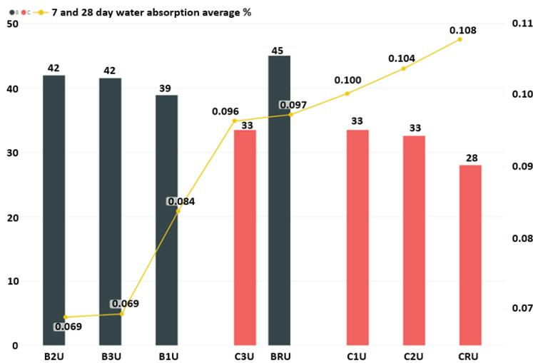
Figure 7. Water absorption-Compressive strength test results of the specimens containing FA.
