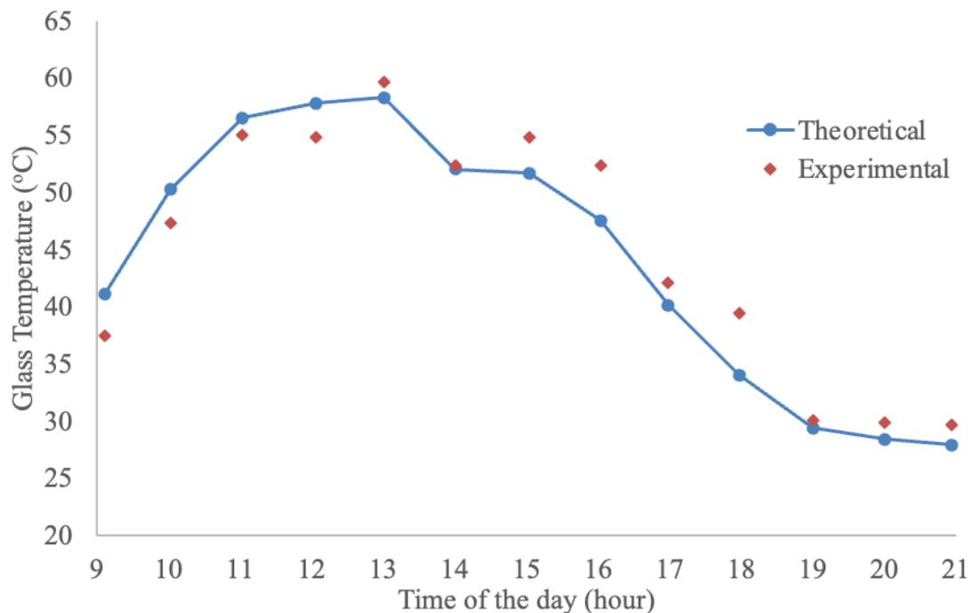
Figure 5. Variation of glass temperature for the basic still.
