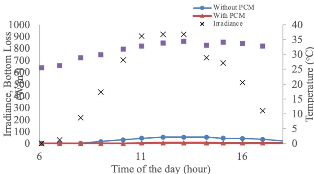
Figure 15. Comparison of bottom losses for the still without and with PCM.
