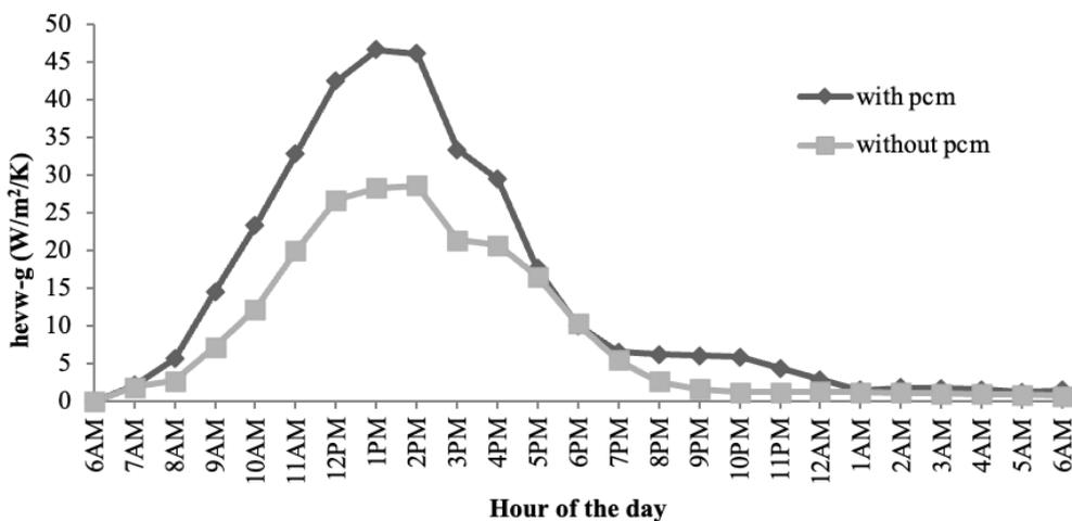
Figure 12. Comparison of the evaporative heat transfer coefficient from water to glass (with and without PCM).
