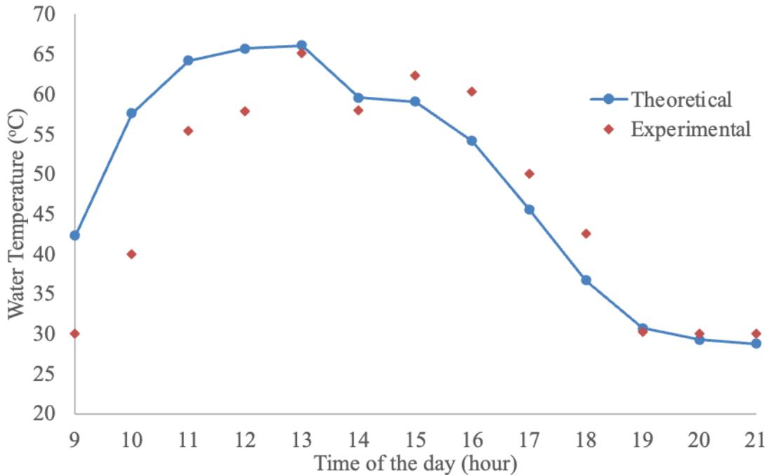
Figure 4. Variation of brackish water temperature for the basic still.
