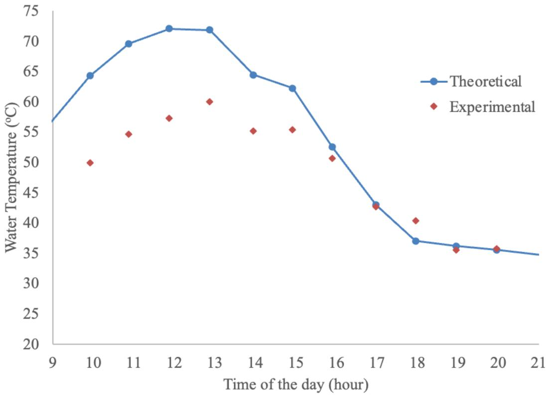
Figure 6. Variation of brackish water temperature for the PCM integrated still.
