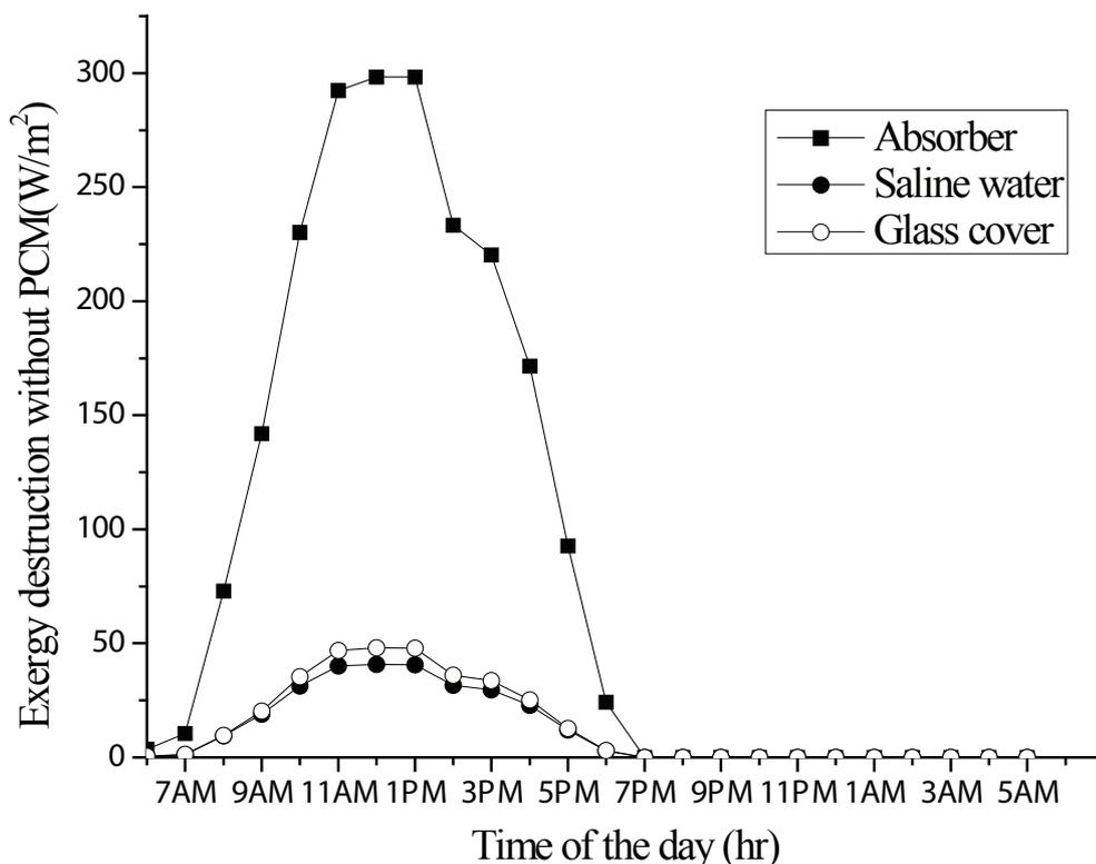
Figure 16. Hourly variation of the exergy destruction in the different parts of the still without PCM.
