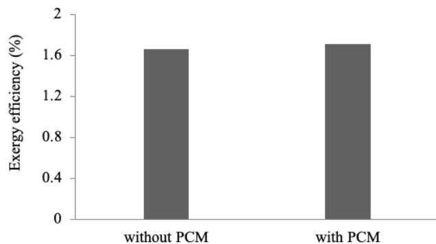
Figure 18. Comparison of the daily exergy efficiencies of the still with and without PCM.
