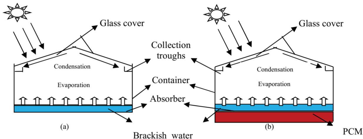
Figure 1. Schematic of (a) basic double slope solar still (b) still with the integration of PCM.
