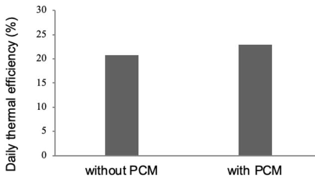
Figure 13. Comparison of the daily thermal efficiencies of the still with and without PCM.
