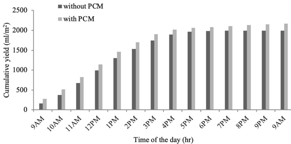
Figure 11. Comparison of the cumulative hourly yield for the still with and without PCM.
