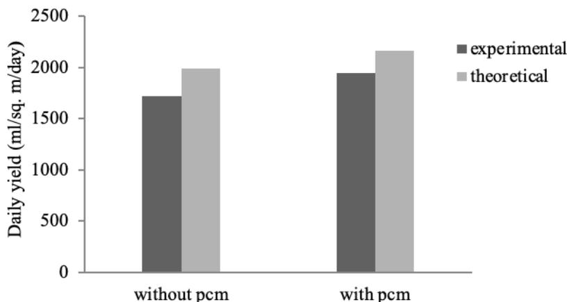
Figure 8. Comparison of yields of the basic still and PCM integrated still.
