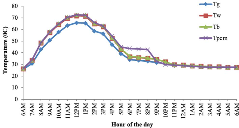
Figure 10. Variation of the temperatures of the still components (PCM integrated still).
