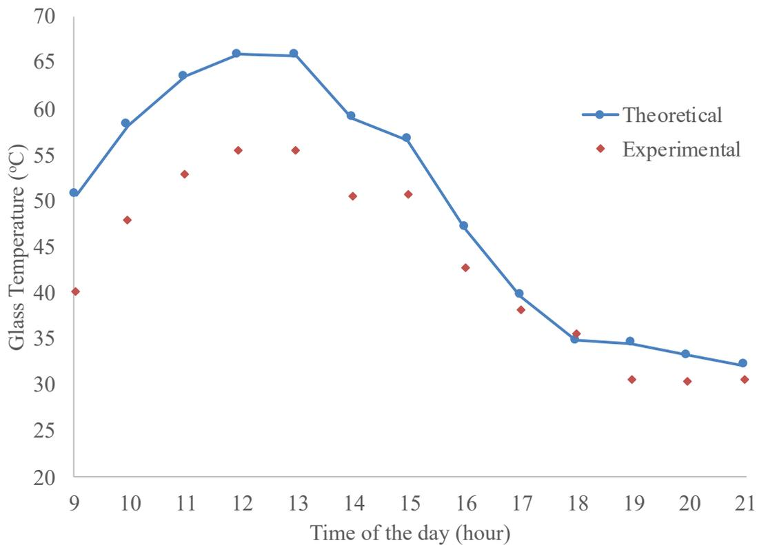
Figure 7. Variation of glass temperature for the PCM integrated still.
