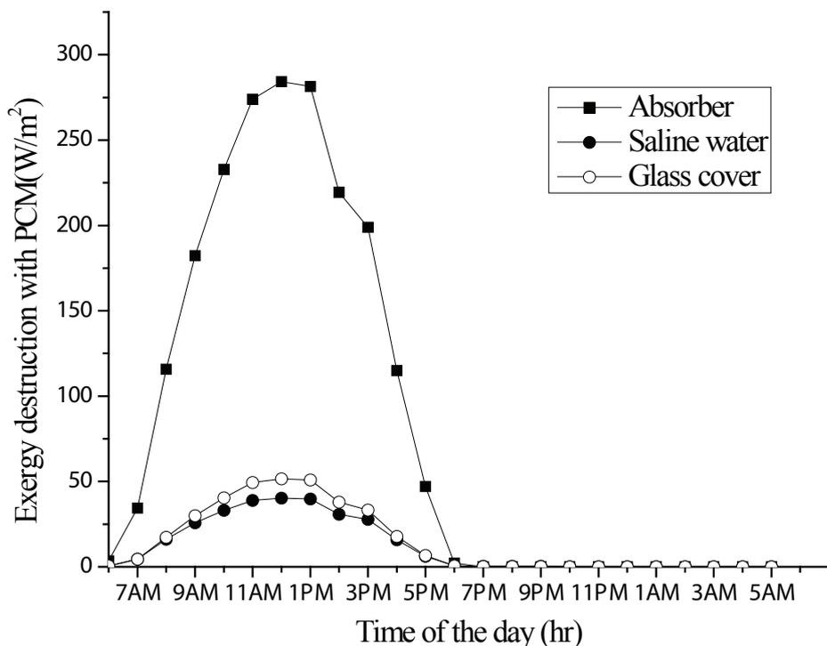
Figure 17. Hourly variation of the exergy destruction in the different parts of the still with PCM.
