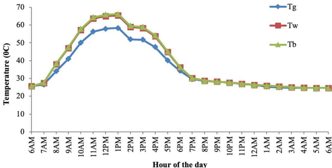
Figure 9. Variation of the temperatures of the still components (basic still).
