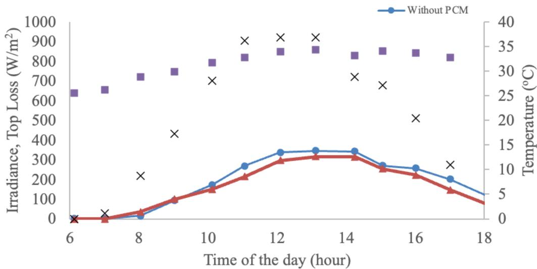
Figure 14. Comparison of top losses for the still without and with PCM.
