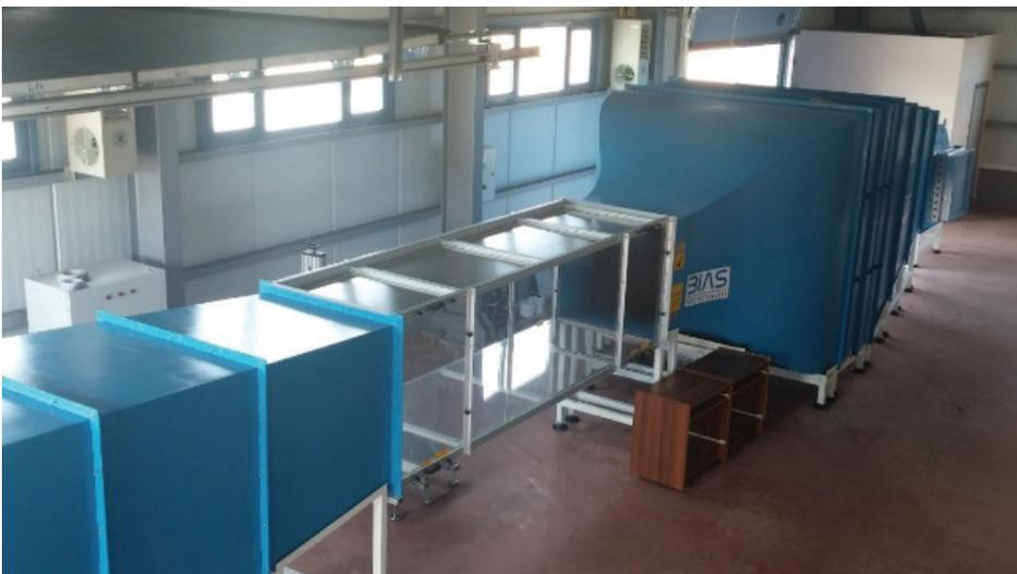
**Figure 2.** Blow down type low speed wind tunnel, the contraction cone and the transparent test section.
