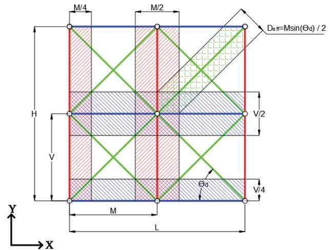
**Figure 4.** Methodology for determining cross-sectional areas of truss elements.
