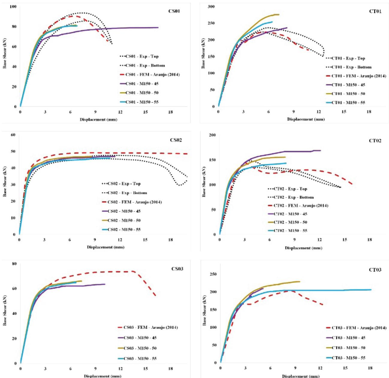
Figure 10. The capacity curves for the 150 mm mesh size.
