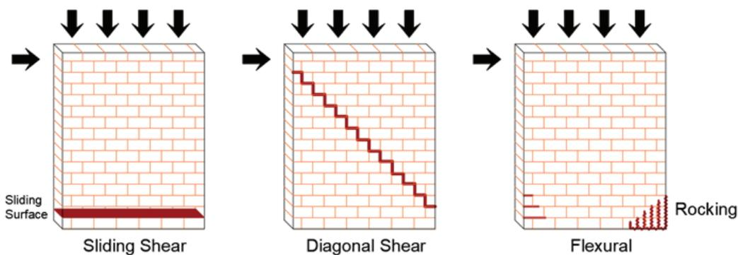
**Figure 1.** Typical failure modes under in-plane loading.
