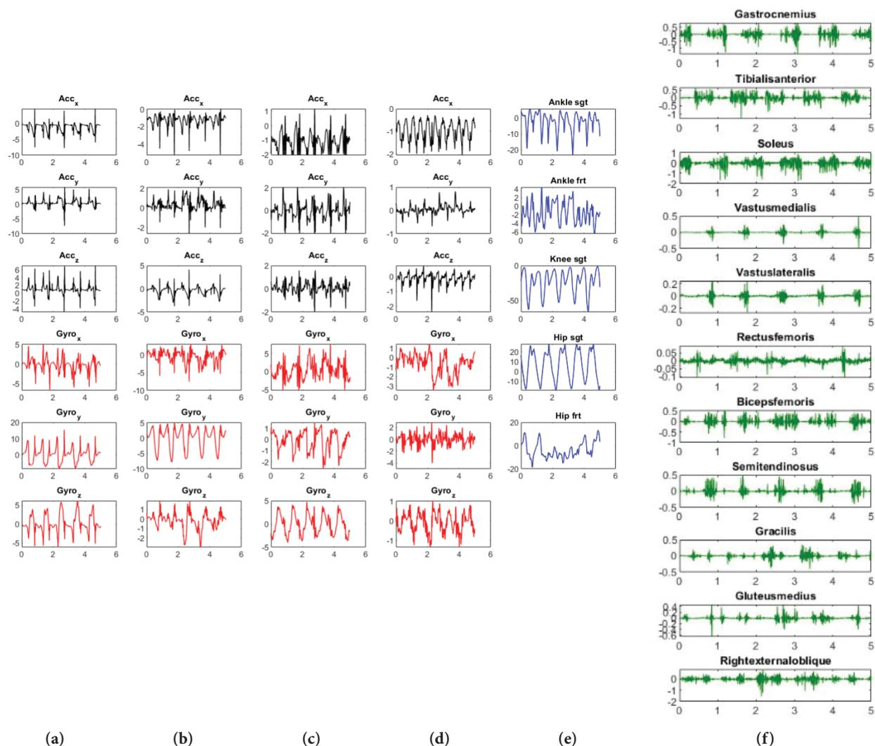
**Figure 2.** Wearable biomechanical sensors time series signal channels. (a) Foot IMU sensor, (b) Shank IMU sensor, (c) Thigh IMU sensor, (d) Trunk IMU sensor, (e) Angles of GON sensor, (f) EMGs of lower extremity muscles.
