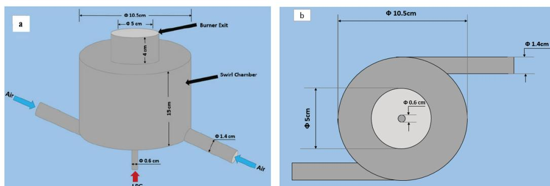
**Figure 4.** Geometrical parameters of the newly created Tangential Swirl Burner a) front view b) top view.
