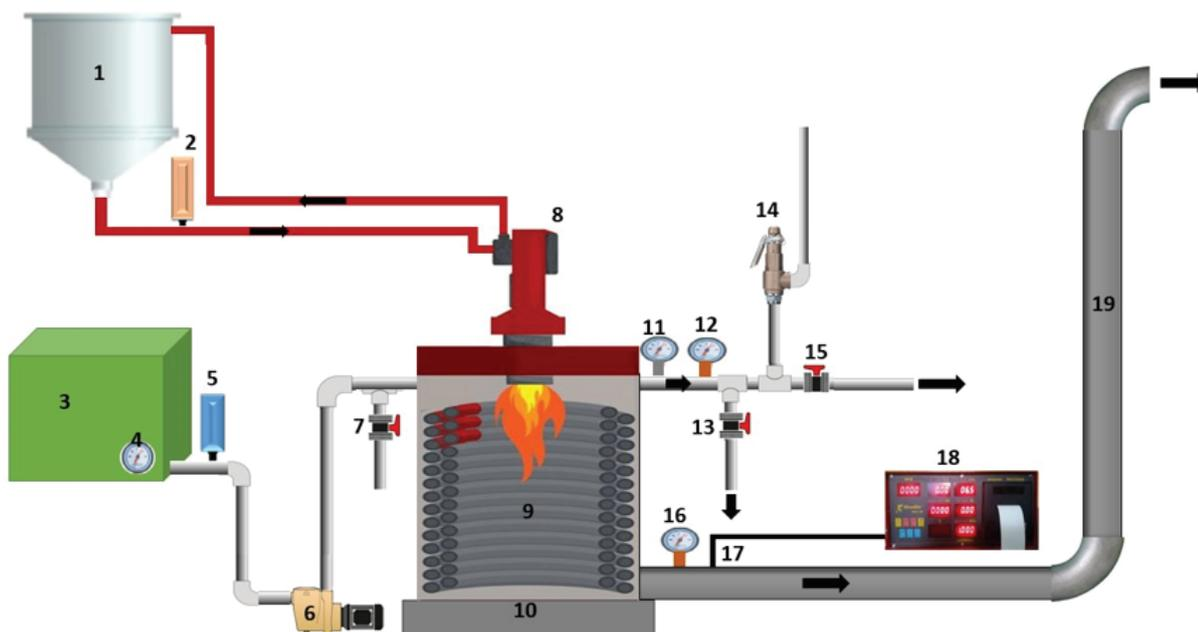
1- Diesel tank, 2- Water tank, 3- Thermometer, 4- Water thermometer, 5- Water flow meter 6- Feed water pump, 7-Draining valve, 8-Diesel burner, 9- Helically coiled tube, 10-Boiler, 11-Pressure gauge, 12- Thermometer, 13- Steam vent valve, 14- Safety valve, 15- Steam supply valve, 16- Exhaust gas thermometer, 17- Exhaust gas analyzer prop, 18- Exhaust gas analyzer, 19- Chimney.
