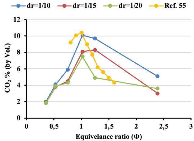
Figure 5. Variation of CO<sub>2</sub> released with exhaust gases at three different diameter ratios.
