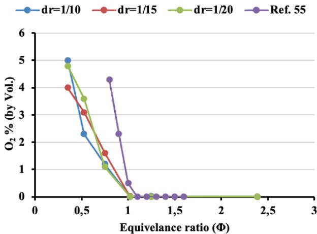
Figure 8 . Variation of O<sub>2</sub> released with exhaust gases at three different diameter ratios.
