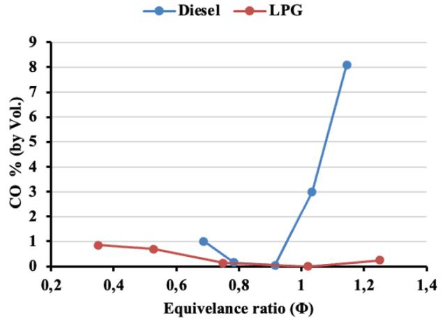
Figure 11. A comparison of CO produced and released by diesel fuel and LPG fuel for dr=1/10.
