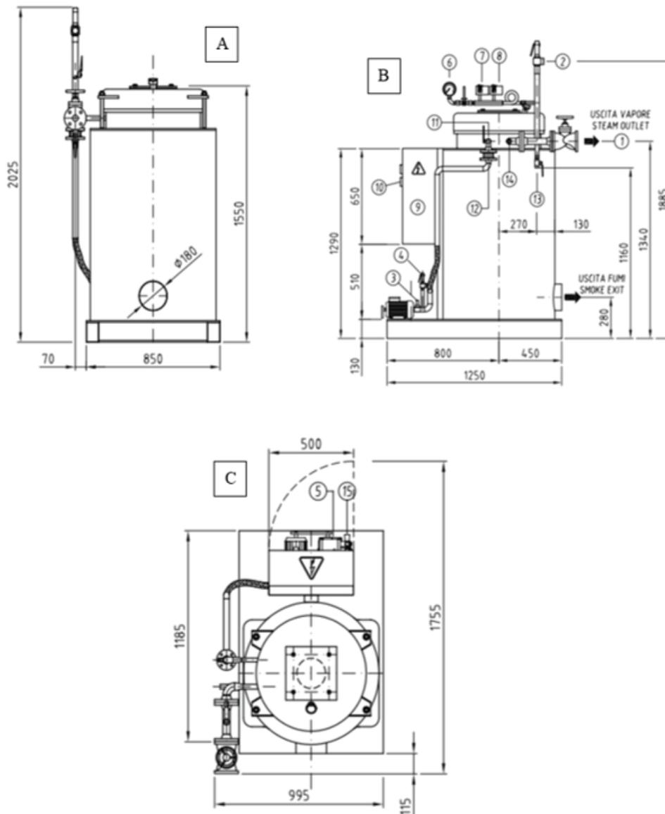
1- steam outlet valve, 2- safety valve, 3- flow switch, 4- overpressure valve outlet, 5- feed water pump, 6- pressure gauge, 7- high to the low pressure switch, 8- safety pressure switch, 9- electric panel, 10- steam thermostat, 11- back washing blow-down, 12- check valve, 13- start-up blowdown, 14- thermostat prop, 15- water inlet.coiled tube, 16- Exhaust gas thermometer, 17- Exhaust gas analyzer prop, 18- Exhaust gas analyzer, 19- Chimney.
