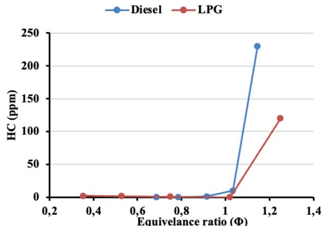
Figure 13. A comparison of HC content with diesel fuel and LPG fuel for dr= 1/10.
