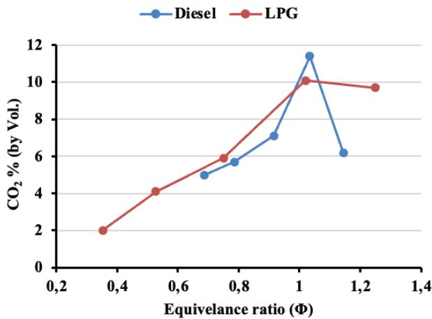
Figure 10. A comparison of CO<sub>2</sub> produced and released by diesel fuel and LPG fuel for dr=1/10.
