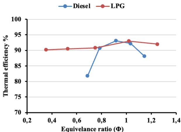
Figure 14. A comparison of boiler efficiency operating with diesel fuel and LPG fuel for  $dr=1/10$ .
