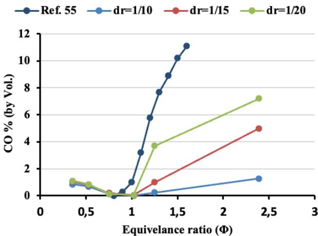
Figure 6. Variation of CO released with exhaust gases at three different diameter ratios.
