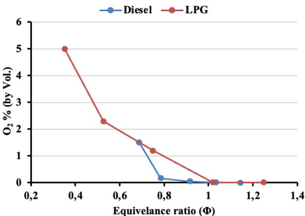
Figure 12. A comparison of O<sub>2</sub> released with diesel fuel and LPG fuel for dr=1/10.
