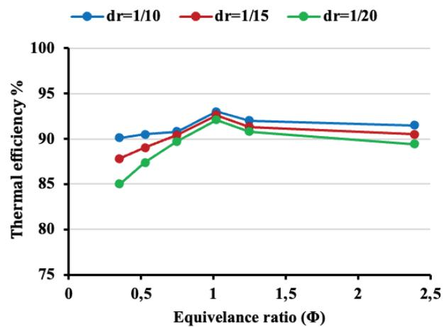
Figure 9. Variation of boiler efficiency with exhaust gases at three different diameter ratios.
