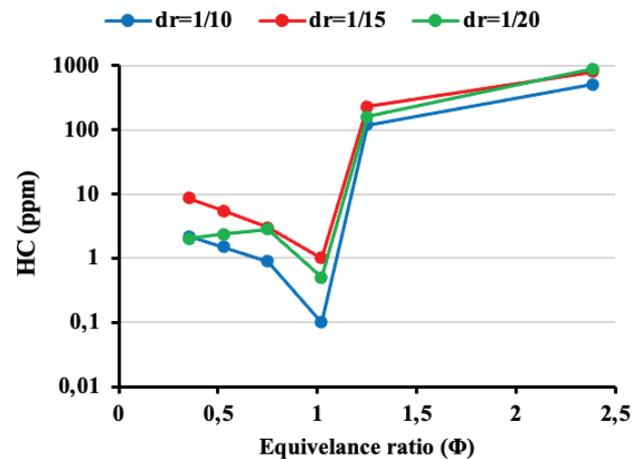
Figure 7. Variation of HC released with exhaust gases at three different diameter ratios.
