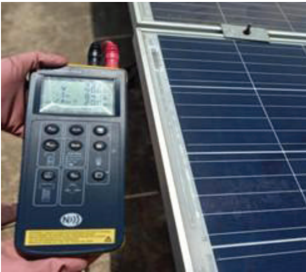
Figure 5. PV200 I-V curve tracer.
