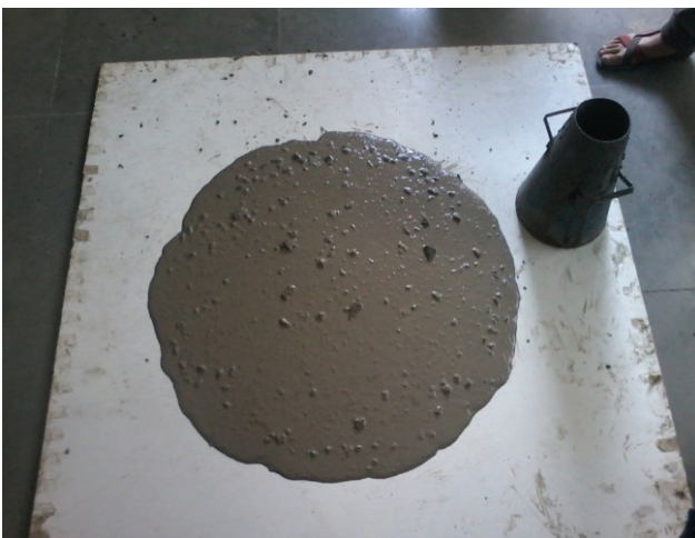
Figure 3. Slump flow of concrete.
