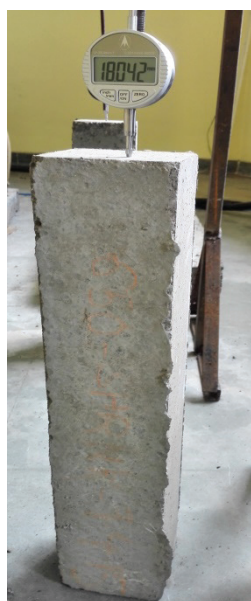
Figure 1. Shrinkage test setup
