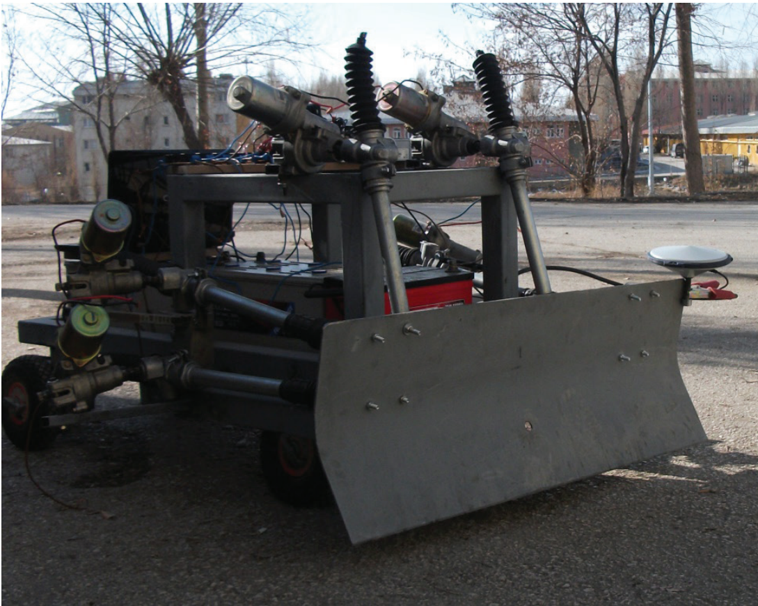
Figure 2. The ready to operate state of the small scale dozer.
