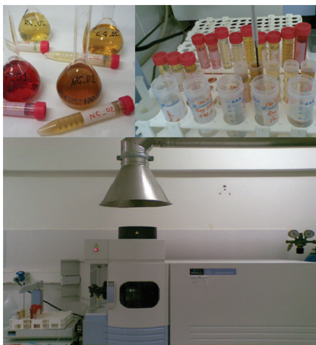
Figure 2. Analysis of element concentration of teas by ICP-OES.
