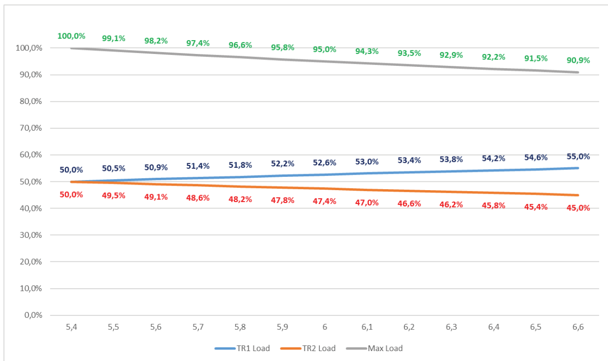
Figure 10. Short-Circuit Voltage Power Load Curve of 5,4 vs 5,4-6,6.
