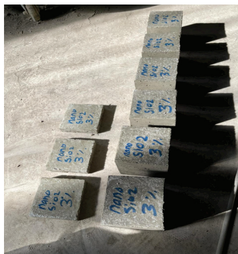
(c) Samples after 28 days extracted from the duration tank
