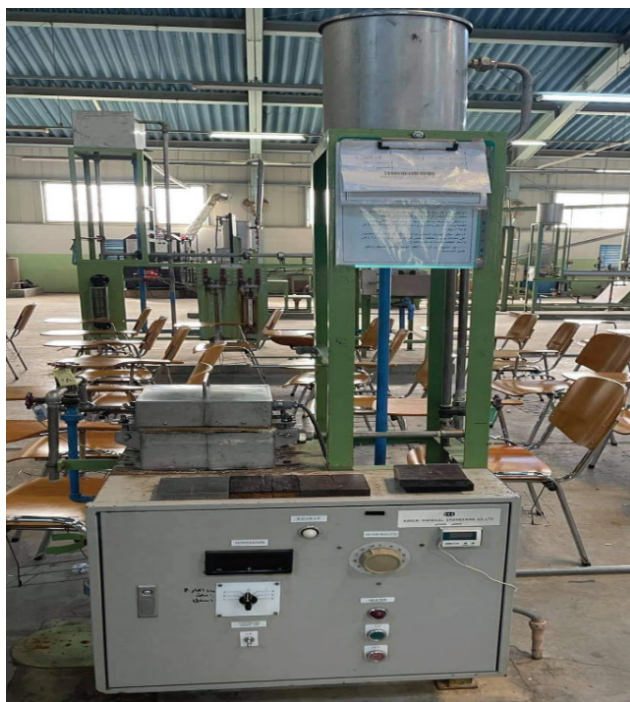
Figure 3. Thermal conductivity device.
