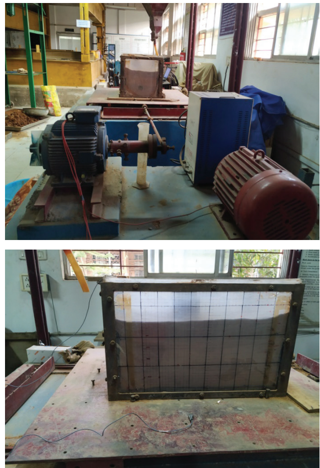
Figure 5. Construction process of model foundation (a) Shake Table set up (b) accelerometer connected at top and bottom of shake table.
