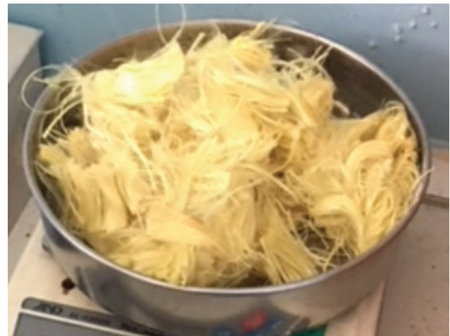
Figure 2. Kevlar fibers added into the mixture.
