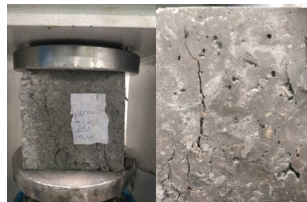
Figure 6. Control sample and PVA-0.15 sample after loading.
