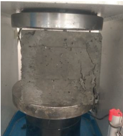
Figure 4. Compression strength test.
