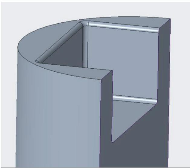
Figure 2. Square cavity chamber.
