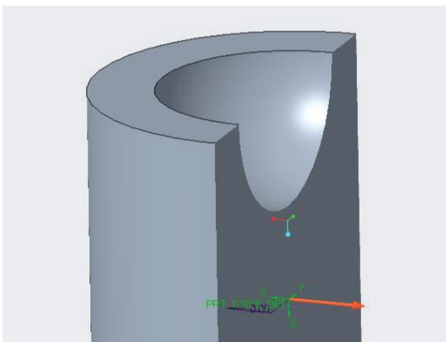
Figure 3. Hemispherical chamber.
