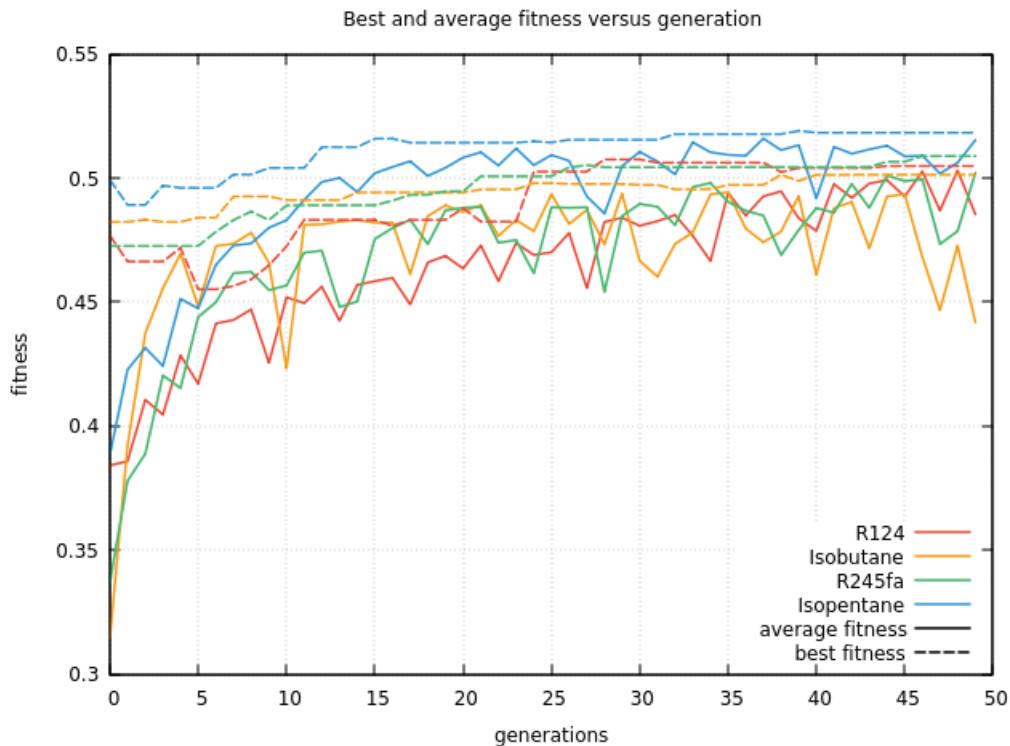
Figure 10. Average and best fitness versus generations for the recuperative supercritical cycle.
