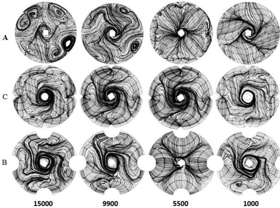
**Figure 8.** Under different Re number, velocity streamlines in three various transverse planes.
