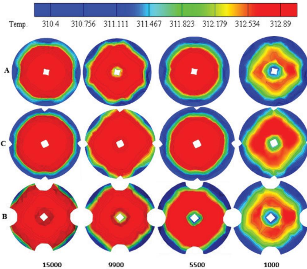
**Figure 9.** The temperature field contour in three various transverse planes in the pipe under different Re numbers.
