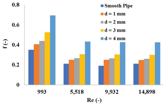
Figure 10. Friction factor variations at different geometrical configurations.
