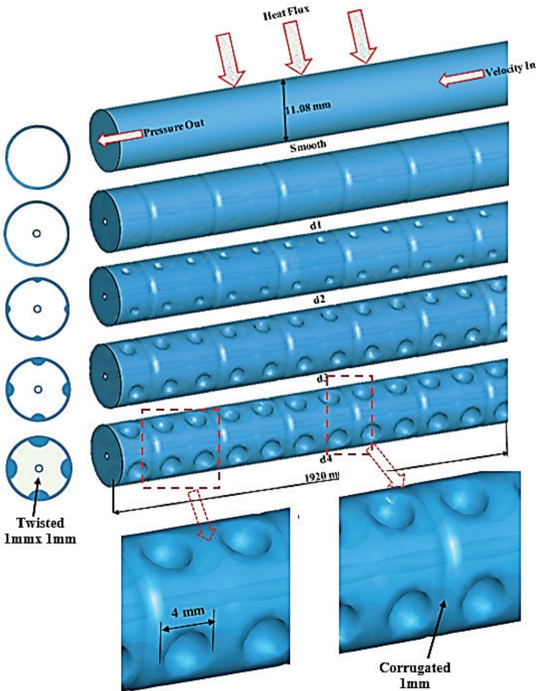
Figure 1. The schematic representation of the 3D domain of plain and modified pipes.
