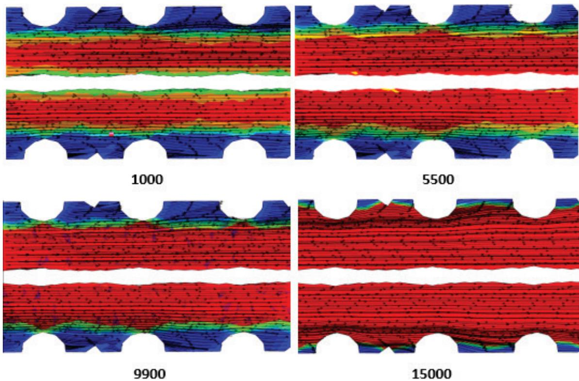
**Figure 5.** Pipe velocity streamlines with different geometrical configurations under various Re numbers.
