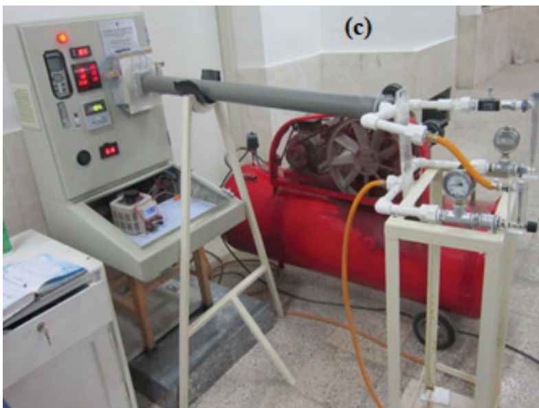
Figure 1. (a) Schematic of the experiment, (b) schematic view of our heat sink with heater, and (c) real photograph of setup.
