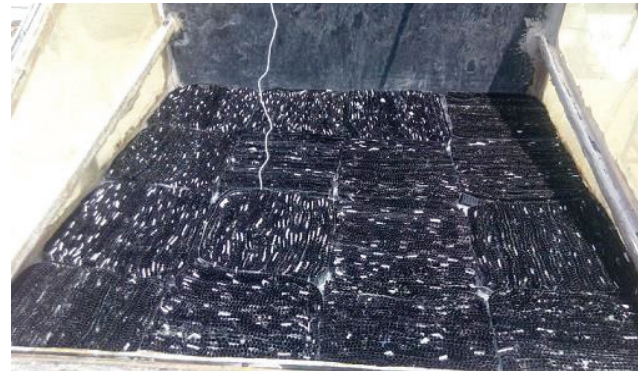
Figure 4. Solar distillation system with honeycomb structure.
