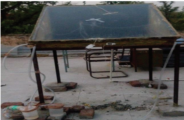
Figure 2. Experimental setup of solar distillation system.
