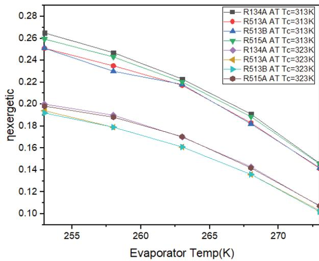
Figure 6. Exergetic efficiency vs Evaporator temperature.
