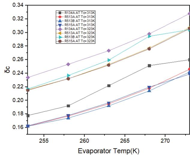
Figure 8. Efficiency defect of condenser vs Evaporator temperature.
