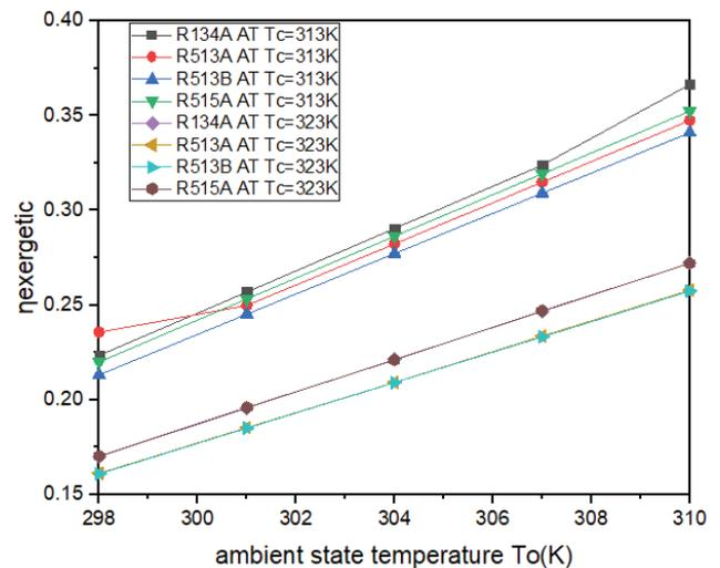
Figure 13. Exergetic efficiency vs Ambient state temperature.
