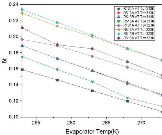
Figure 10. Efficiency defect in throttle valve vs Evaporator temperature.
