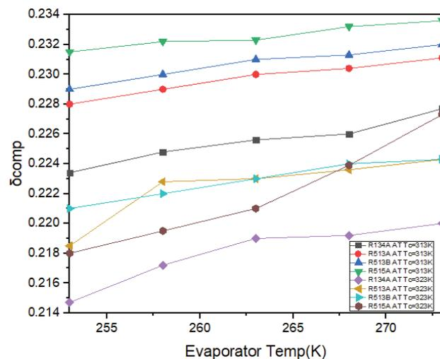
Figure 12. Efficiency defect of Compressor Vs Evaporator temperature.
