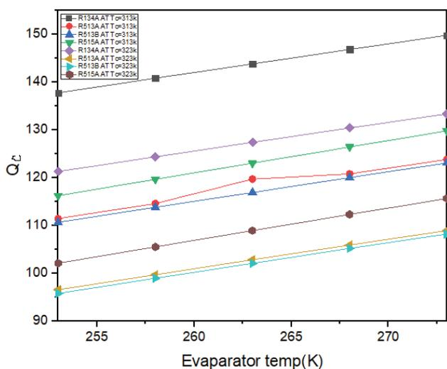
Figure 4. Cooling capacity Vs Evaporator temperature.
