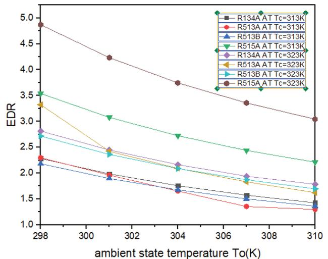
Figure 14. EDR vs Ambient state temperature (at  $T_E = 273K$ ).
