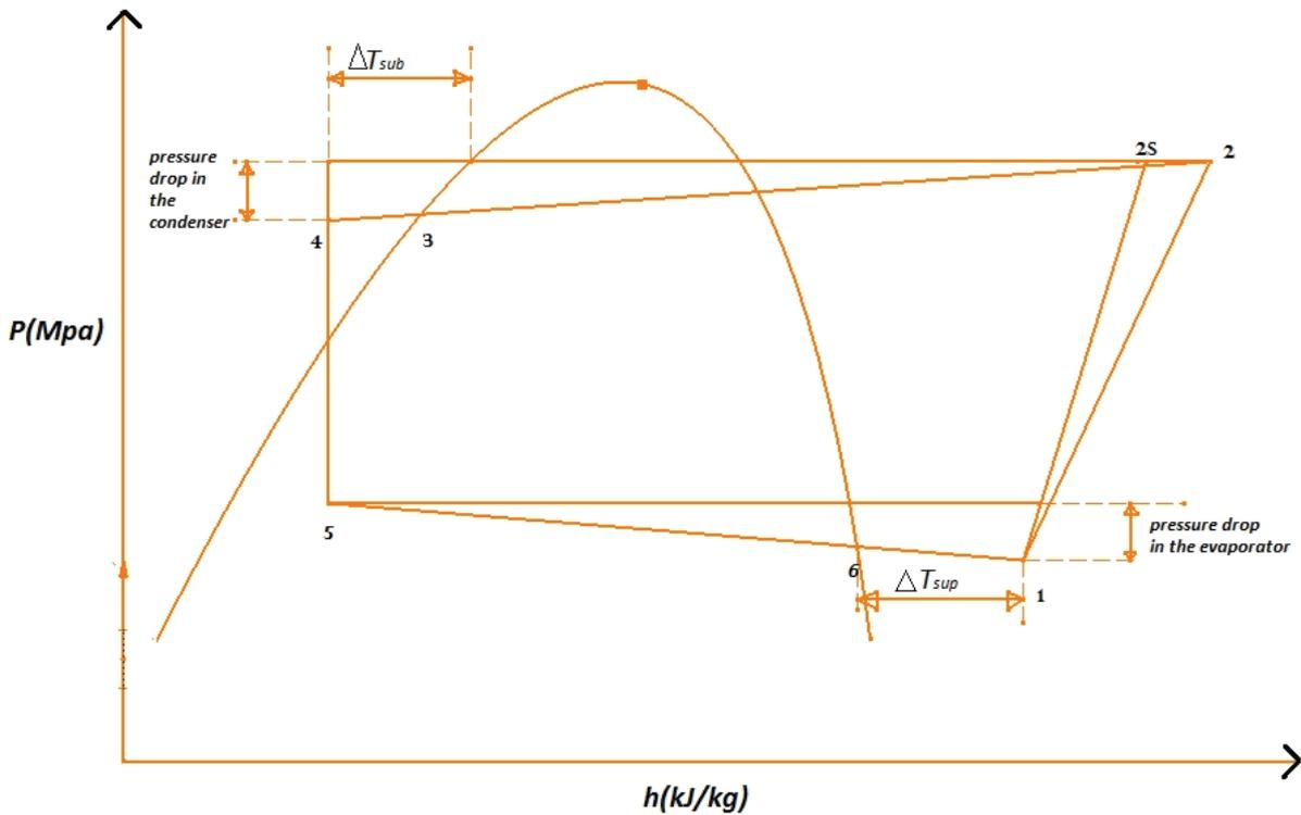
Figure 2. Pressure-enthalpy diagram of a refrigerator with LSHX.
