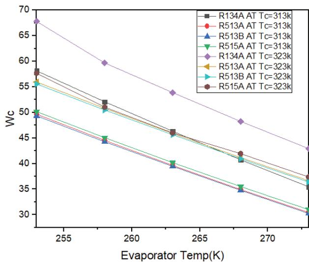
Figure 3. Compressor power consumption vs Evaporator temperature.
