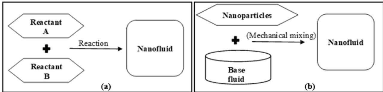
**Figure 1.** (a) One-step method, (b) Two-step method of nanofluid preparation.
