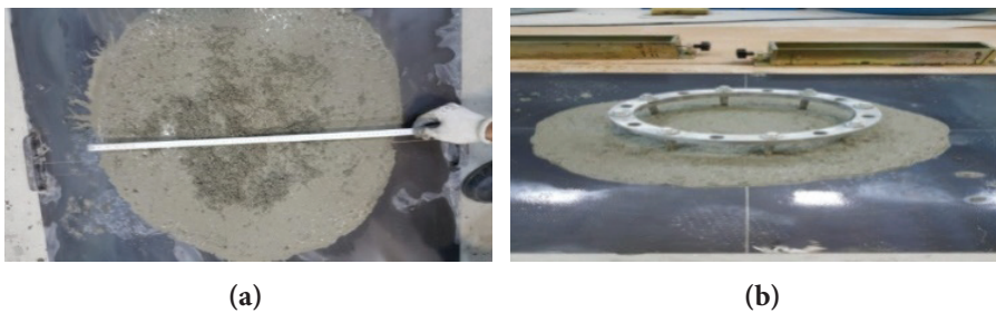
Figure 3. The slump-flow and J-ring tests for MIC0.25 mixture.
