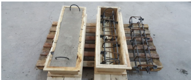
Figure 5. Casting position and reinforced bar details.
