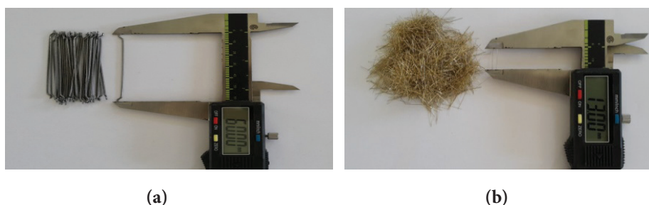
Figure 2. Shape of macro and micro fibers used in the mixtures.
