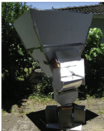
Figure 9. Non-imaging concentrator based reflective solar cooker [68].
