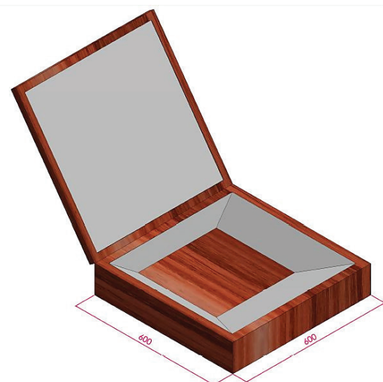
Figure 4. Assembly drawing of new designed solar cooker.
