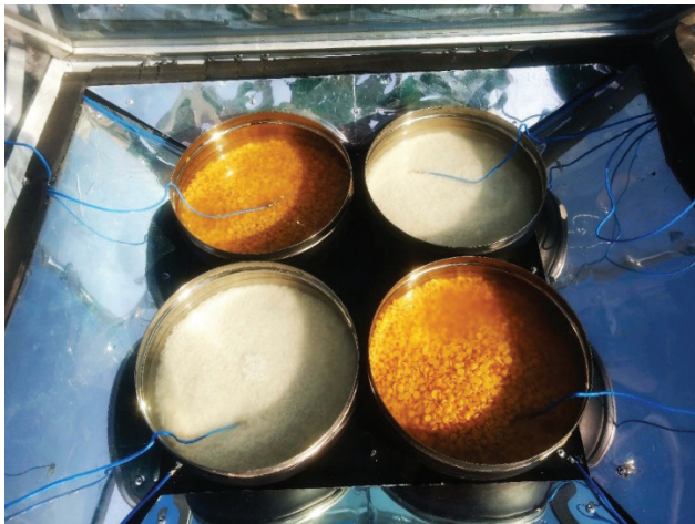
Figure 11. Daal and rice placed in new designed Solar Cooker for cooking.
