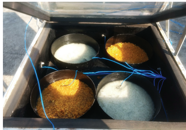
Figure 10. Daal and rice placed in commercial Solar cooker for cooking.
