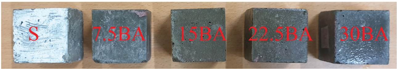
Figure 12. Visual inspection over 10 months after magnesium sulfate effect.
