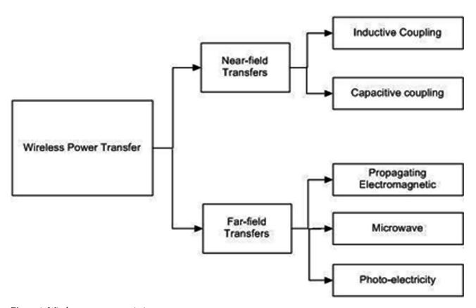
Figure 1. Wireless power transmission types.
