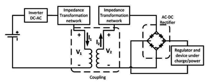
Figure 2. Typical near-field power transfer system structure.
