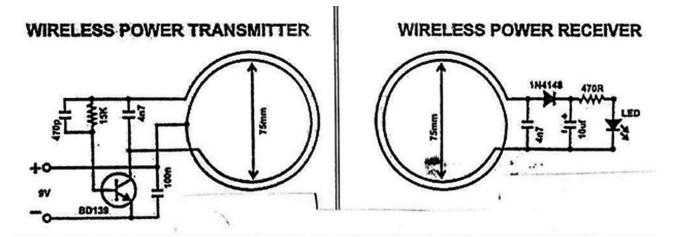
Figure 6. Circuit diagrams of Wire Power Transmitter and Receiver.
