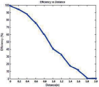
The voltage transmitted to receiver drops because there is increase in the distance between the transmitter and receiver. The efficiency of the power transmitted drops because there is increase in the distance between transmitter and receiver.
