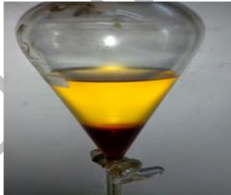
Figure.3 Transesterification of watermelon biodiesel
