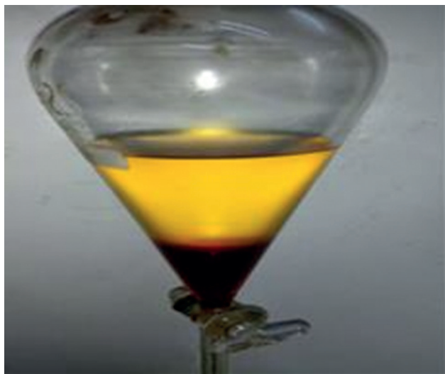
Figure 3. Transesterification of watermelon biodiesel.
