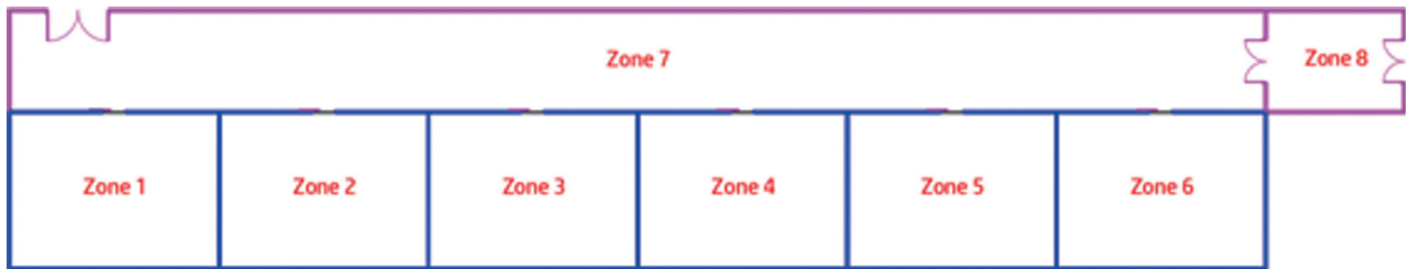
Zones 1→6: Cold rooms (Area of each room: 180 m 2 ; Height: 7.8 m); Zone 7: Corridor (Area: 540 m 2 ; Height: 5 m); Zone 8: Loading dock for trucks (Area: 36 m 2 ; Height: 5 m)
