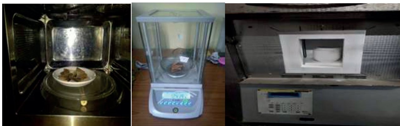
Figure 2. Wood chips placed inside microwave oven for drying, weighing and crucible inside a muffle furnace.
