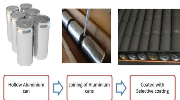
Figure 1. Process of making solar collector from waste cans.
