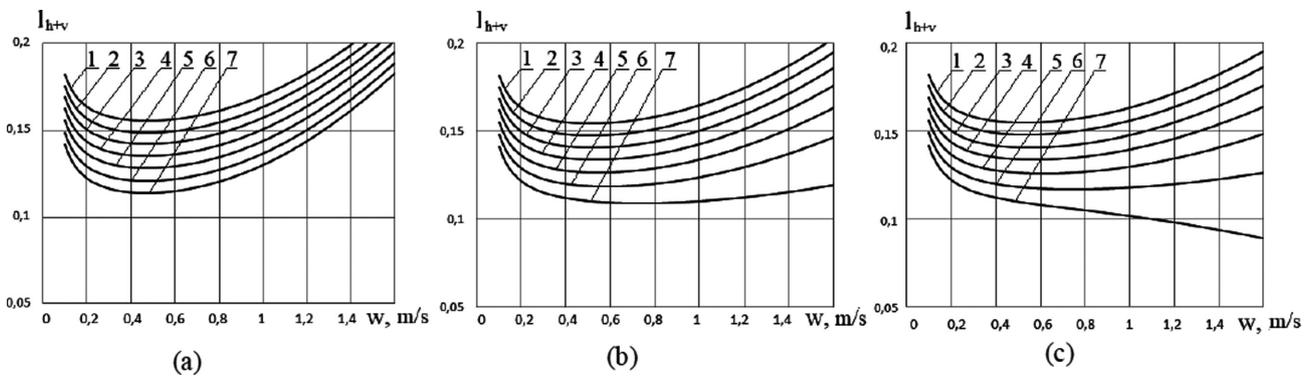
**Figure 4.** The dependence of the total consumption of external energy for heating and ventilation system from the coolant velocity in lower circuit: (a)  $K^e = 0$ , (b)  $K^e = 0,2$ , (c)  $K^e = 0,3$ ; 1 – 7 –  $t_0 = -20 \dots 10$  °C.
