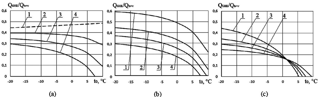
**Figure 7.** The dependence of the specific load of ground heat exchanger from the temperature of the air: a) 1 – 4 –  $K^c = 0 \dots 0,3$ ; b) 1 – 4 –  $\eta_r = 0.0, 0,8$  c) 1 – 4 –  $m = 0 \dots 2$ .
