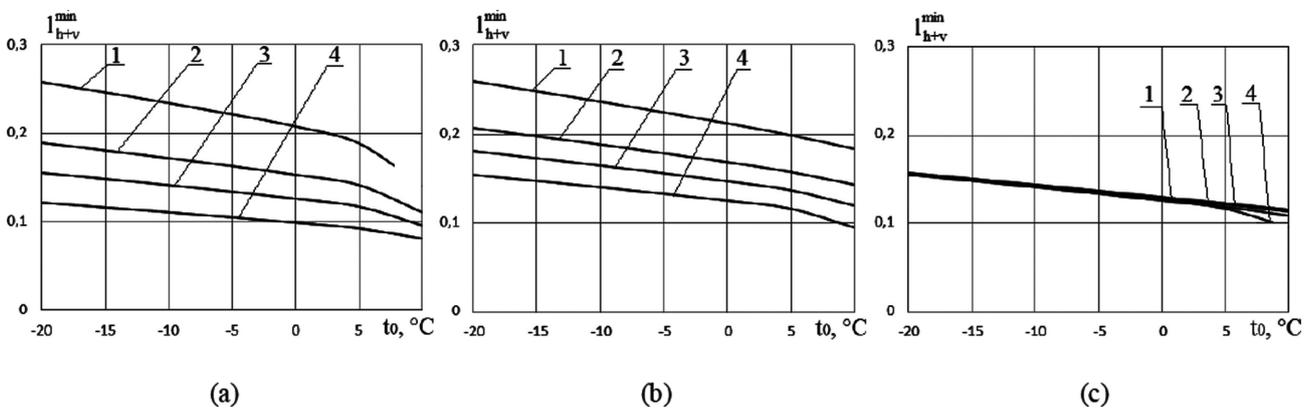
Figure 6. The dependence of the minimal unit consumption of external energy for system from the temperature of atmospheric air: (a)  $1 - 4 - m=0...2$ ; (b)  $1 - 4 - \eta_r=0...0,8$ ; (c)  $1 - 4 - K^e=0...0,3$ .
