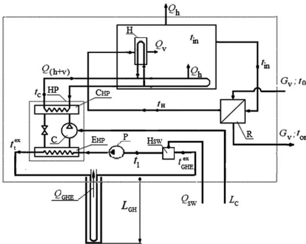
**Figure 1.** Schematic diagram of the combined heating and ventilation system based on ground heat pump with the additional using of heat of ventilation emissions and wastewater: HP–heat pump;  $C_{HP}$  – condenser;  $E_{HP}$  – evaporator; C – compressor;  $H_{sw}$  – heat exchanger for recover heat of sewage water; H–heater of fresh air; P – pump; R – recuperator.
