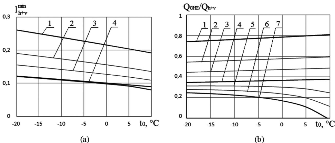
**Figure 8.** The dependence of the minimal specific energy consumption and the specific load of the ground heat exchanger from the temperature of atmospheric air: a) 1 –  $m = 0 \dots 2$ ; 1 – 4 –  $K^c = 0$  ( $\eta_r = 0; 0,4; 0,6; 0,8$ ); 4 –  $K^c = 0 \dots 0,3$ ; b) 1 –  $m = 0 \dots 2$ ; 1 – 4 –  $K^c = 0$  ( $\eta_r = 0; 0,4; 0,6; 0,8$ ); 5 – 7 –  $K^c = 0 \dots 0,3$ .
