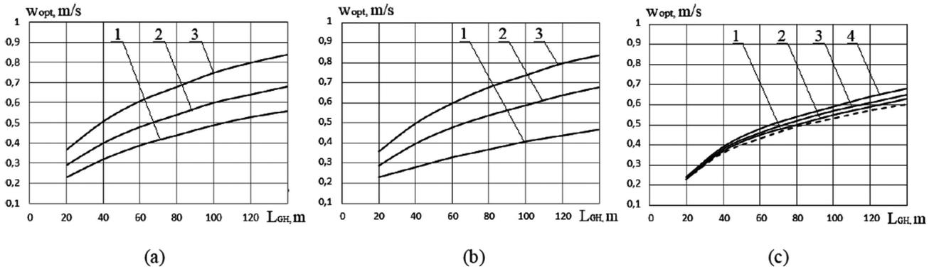
**Figure 3.** The dependence of the optimal coolant velocity in lower circuit from the depth of well: (a) 1 – 3 –  $d_{in} = 0,04; 0,032; 0,025$  m accordingly; (b) 1 – 3 –  $q_G = 25; 50; 75$  W/m accordingly; (c) 1 – 4 –  $K^e = 0; 0,1; 0,2; 0,3$  accordingly.
