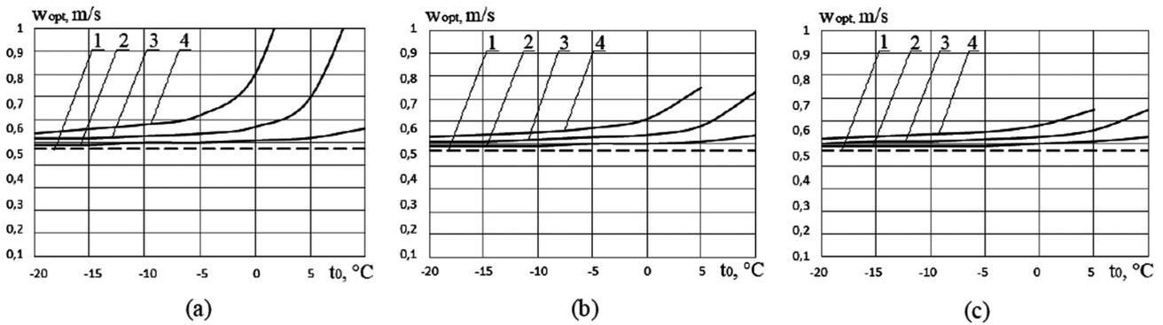
Figure 5. The dependence of the optimal coolant velocity in lower circuit from the temperature of atmospheric air: (a)  $m=0$ , (b)  $m=1$ , (c)  $m=2$ ;  $1 - 4 - K^e=0...0,3$ .
