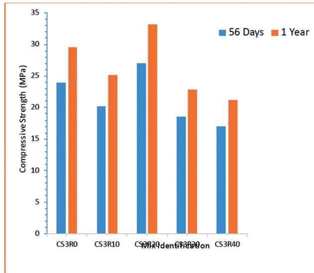
**Figure 2.** The 56 and 365 days compressive strength results.
