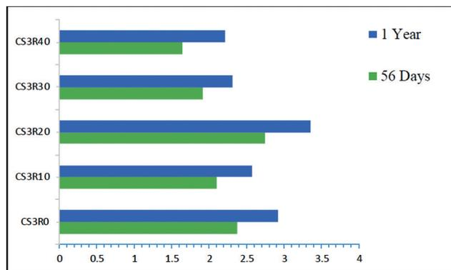
**Figure 3.** The 56 and 365 days splitting tensile strength results.
