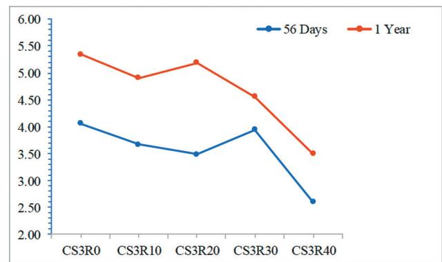
**Figure 4.** The 56 and 365 days flexural strength test results.
