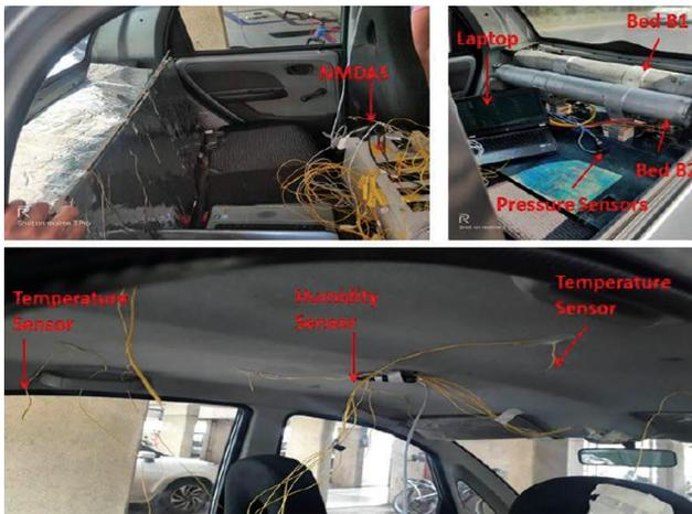
Figure 13. Instrumentation of NMDAS in vehicle.
