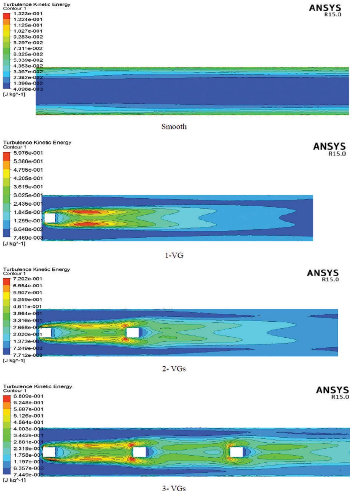
Figure 12. The contours of turbulence kinetic energy (BR = 0.2) for different VGs number.
