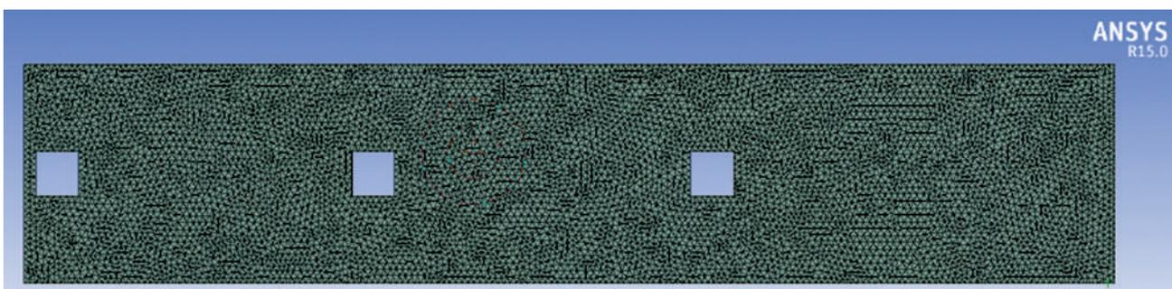
Figure 4. Side view of the meshed test region.
