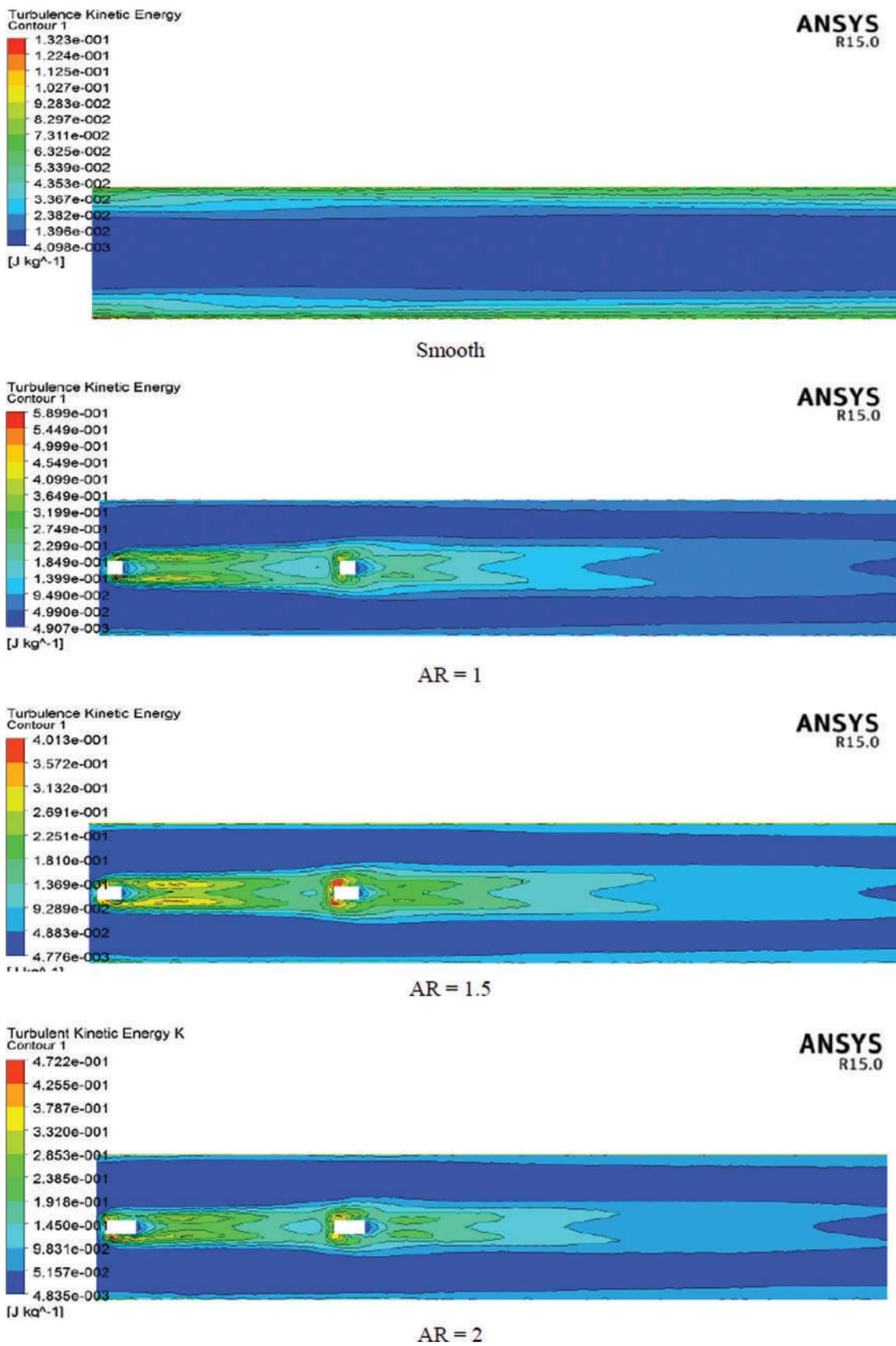
Figure 21. The contours of turbulence kinetic energy for different aspect ratio (BR=0.1, 2-VGs)
