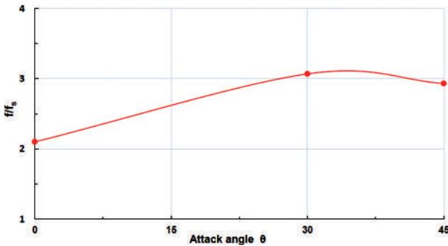
Figure 17. Variation of friction factor with attack angle (BR = 0.2, VGs = 3).
