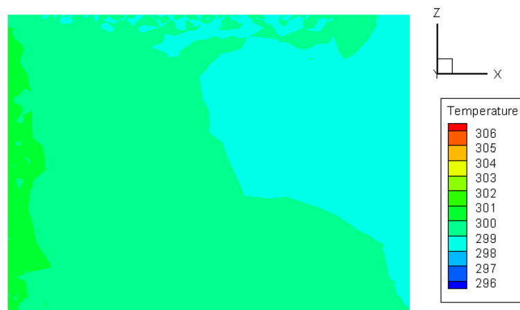
Figure 11. Temperature contours in horizontal plan of the proposed room with natural convection
