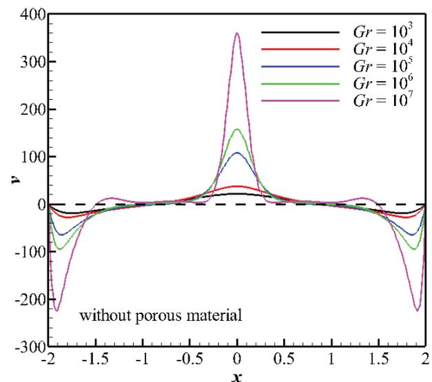
**Figure 9.** Vertical velocity distribution along  $x$  in the middle of the cavity above the cylinder at  $y = 1.25$ , for different Grashof numbers without the presence of porous material.
