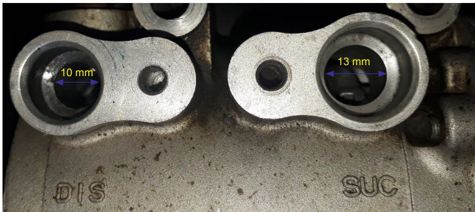
Figure 4. Discharge and suction port diameters of selected scroll compressor.
