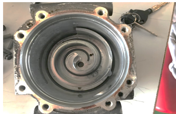
Figure 3. Selected scroll compressor (Left side) and inside view of scroll compressor (Right side).
