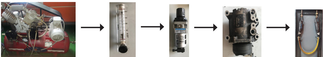
1 – Air Compressor, 2 – Air flow meter, 3 – Air filter with pressure regulator, 4 – Scroll compressor, 5 – Mechanical load
